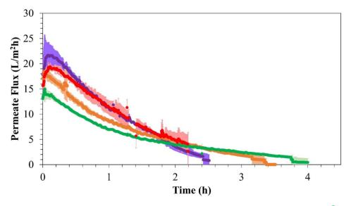
Fig. 2 Permeate fluxes during reverse osmosis concentration of model solution at transmembrane pressures of ( ) 2.5, ( ) 3.0, and ( ) 3.5 MPa, and ( $\bigcirc$ ) cranberry juice at 3.5 MPa. Values presented are mean  $\pm$  standard deviation.
