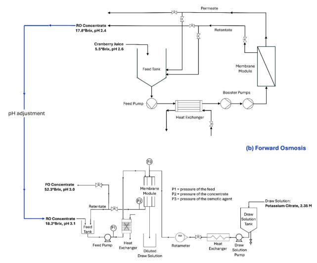
Fig. 1 Schematic diagram of (a) reverse osmosis<sup>46</sup> and (b) forward osmosis concentration processes
