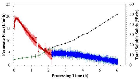
Fig. 3 Permeate flux and total soluble solids content (TSSC) during reverse osmosis (RO) and forward osmosis concentration of cranberry juice. Values presented are mean  $\pm$  standard deviation. ( RO) RO flux; ( FO) TSSC during RO; ( TSSC during FO).
