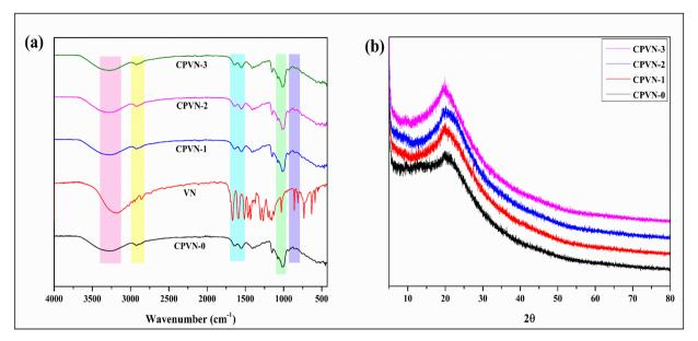
Fig. 3 (a) FTIR spectra and (b) XRD pattern of control CPVN and active films.
