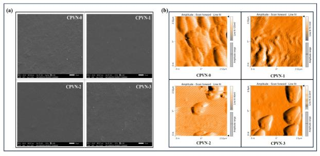
Fig. 4 (a) SEM and (b) AFM micrographs of control CPVN and active films.
