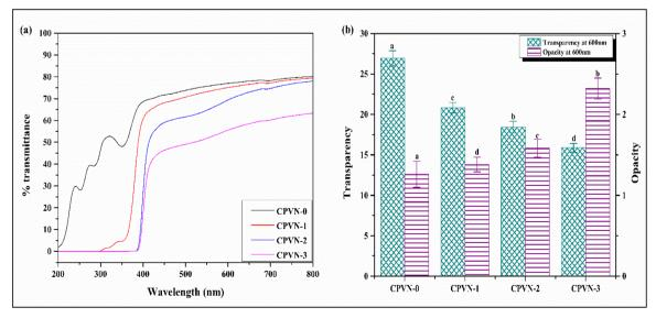
Fig. 2 (a) % Transmittance (b) transparency and opacity of control CPVN and active films
