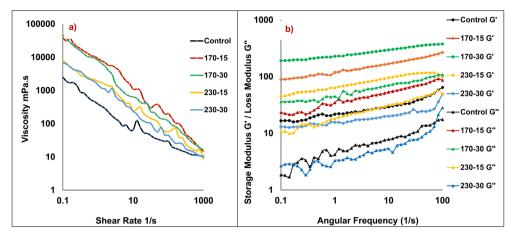
Fig. 3 Effect of cold plasma on (a) steady shear and (b) oscillatory – frequency dependent rheological characteristics of oat protein dispersions.
