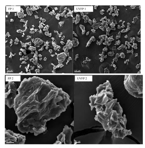
Scanning electron microscope images of FP (1 and 2 at  $110 \times$  and  $655 \times$  respectively) and UVFP (1 and 2 at  $110 \times$  and  $885 \times$  respectively).
