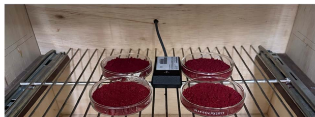
Fig. 2 UVFP samples placed in the UV-C chamber for treatment with UV-C radiation.
