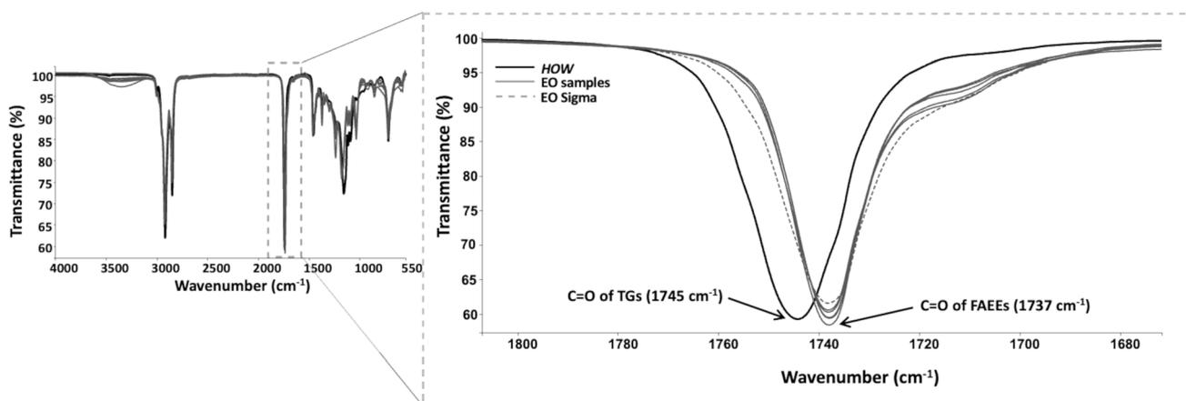
Fig. 2 FTIR-ATR spectra represented in absorbance of all EO samples synthesized, EO Sigma (commercial) and High Oleic Waste (HOW).
