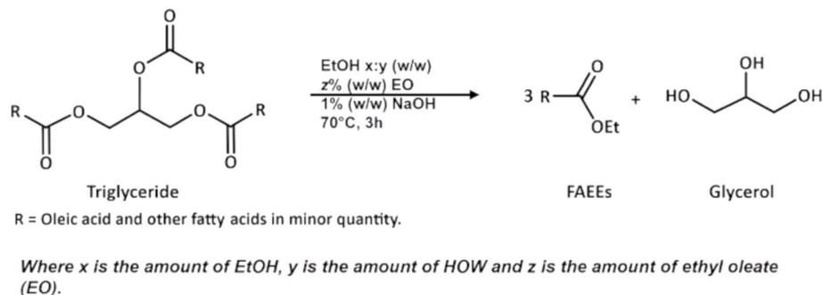
Fig. 1 Schematic representation of the synthesis of FAEEs, namely ethyl oleate by the transesterification reaction of a triglyceride with ethanol.
