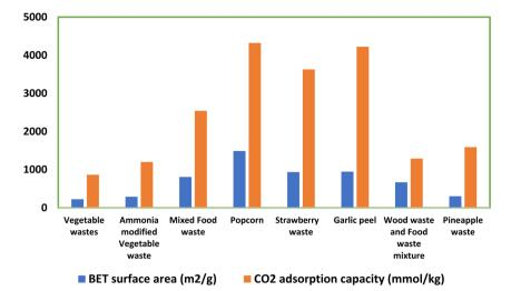
Fig. 3 CO<sub>2</sub> adsorption using food waste biochar. <sup>23,91,93–97</sup>
