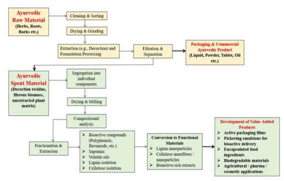
Fig. 4 Process flow of Avurvedic product preparation and valorisation of spent materials into bioactives and value-added products.
