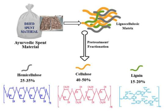
Schematic of lignocellulosic biomass components derived from Ayurvedic spent materials (Adopted from Abraham et al. 40)
