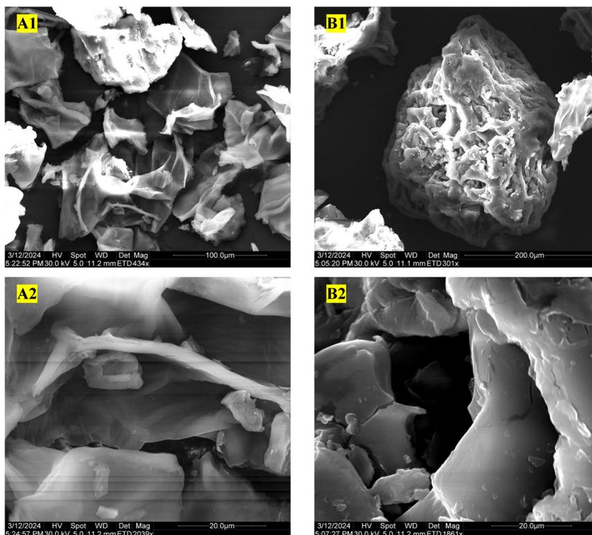
**Fig. 2** Scanning electron microscopy (SEM) images of pomelo peel (PP) particles of different sizes, with 125  $\mu\text{m}$  PP particles shown at 400 $\times$  magnification (A1) and 2000 $\times$  magnification (A2) and 250  $\mu\text{m}$  PP particles at 300 $\times$  magnification (B1) and 1800 $\times$  magnification (B2); the scale bars represent 100  $\mu\text{m}$  (A1), 20  $\mu\text{m}$  (A2), 200  $\mu\text{m}$  (B1), and 20  $\mu\text{m}$  (B2).
