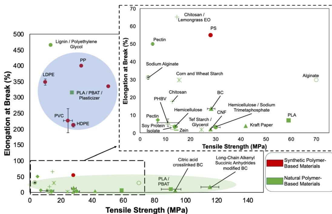
Fig. 3 The comparison of tensile strength and elongation at break of different film-based materials.<sup>83,98,172–195</sup>
