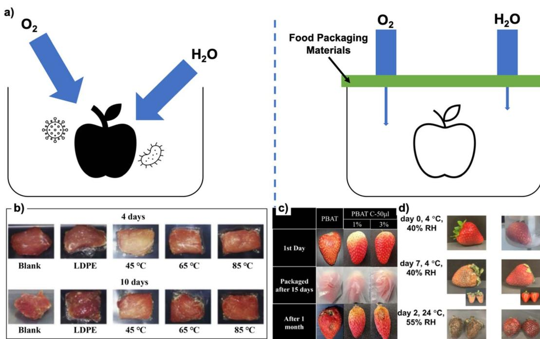
Fig. 4 (a) The use of food packaging materials to prevent quality changes in food, and the example of using (b) chitosan-based<sup>200</sup> (Reprinted with permission from MDPI), (c) PLA<sup>201</sup> (Reprinted with permission from Springer Nature), and (d) bacterial cellulose-based food packaging materials<sup>85</sup> (Reprinted with permission from American Chemical Society).
