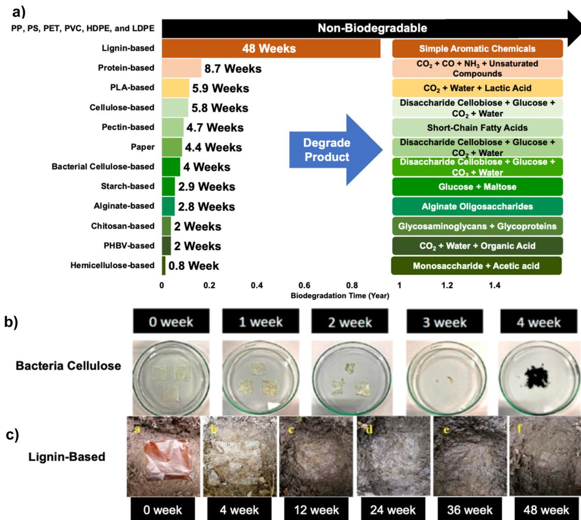
Fig. 5 (a) Biodegradation time of different FPMs,<sup>10,26,82,111,178,179,250–263</sup> (b) degradation of bacterial cellulose<sup>264</sup> (Reprinted with permission from MDPI), and (c) degradation of lignin-based films<sup>255</sup> (Reprinted with permission from Elsevier).
