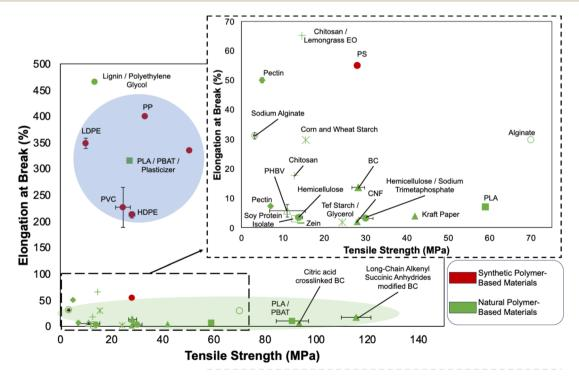
The comparison of tensile strength and elongation at break of different film-based materials. 83,98,172-195
