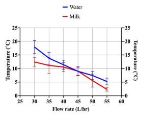
Fig. 8 Experimental results showing temperature increase for milk and water during single-pass heating trials at varying flow rates (30-55 L h<sup>-1</sup>) using the fabricated PTC system, highlighting the effect of flow rate on thermal performance.
