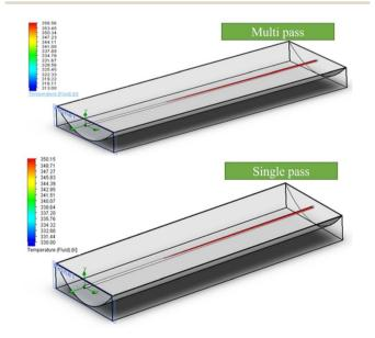
Fig. 6 Simulation results for milk heating at a flow rate of 30 L  $h^{-1}$  using the optimized PTC configuration, showing predicted inlet and outlet temperatures under both multi-pass and single-pass operation.
