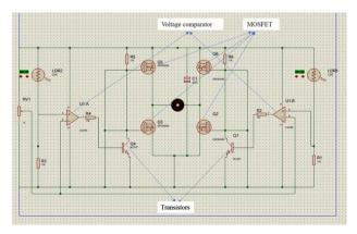
Fig. 3 Circuit diagram of the developed single-axis solar tracking system, illustrating the configuration of light-dependent resistors (LDRs), voltage comparator (LM358), H-bridge motor driver, and associated electronic components
