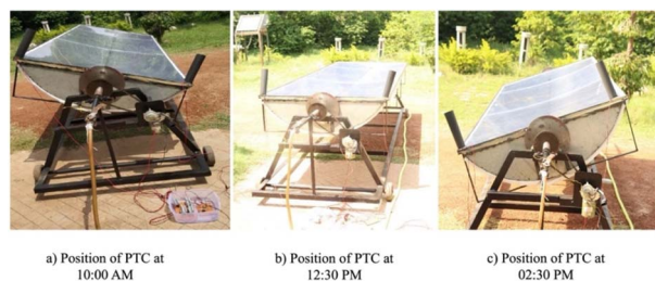
Fig. 5 Sequential images showing the position and movement of the PTC system throughout the day under the control of the developed solar tracker, capturing east-to-west sun tracking between 10:00 AM and 2:30 PM.
