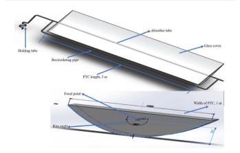
Fig. 1 Dimensional schematic of the parabolic trough collector (PTC) showing the major components, including the reflector, receiver tube, support structure, and alignment details.
