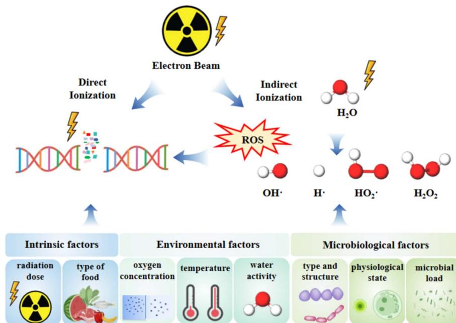
Fig. 2 The mechanism of EBI inactivation technology.
