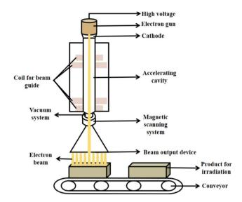
Schematic diagram of the electron accelerator.
