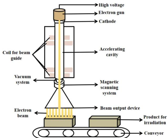
Fig. 1 Schematic diagram of the electron accelerator.
