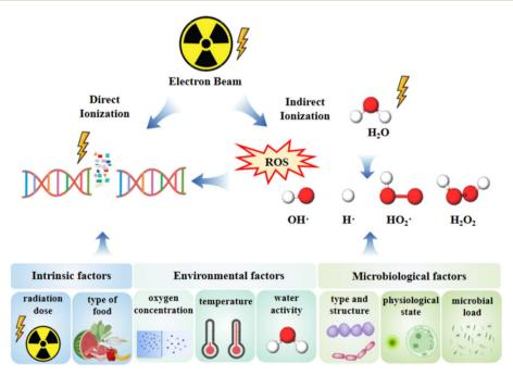
Fig. 2 The mechanism of EBI inactivation technology
