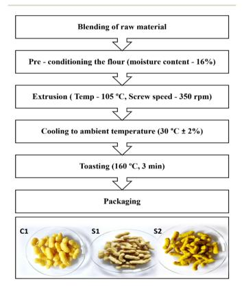
Fig. 1 Flowchart of the extrusion process for producing EPS: C1 – control, S1 - EPS with blended flour, and S2 - EPS with lignin-based Pickering emulsion (LPE) fortification.
