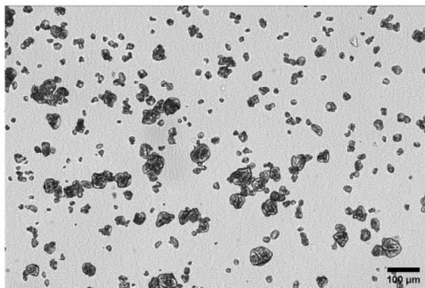
Fig. 2 Light microscopy of typical spray dried particles.
