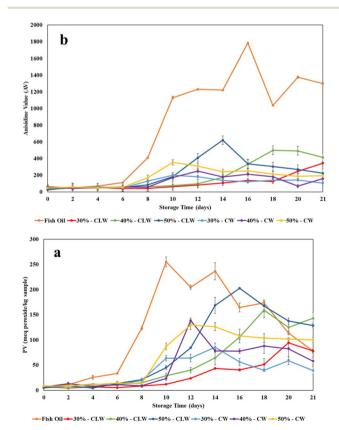
Fig. 6 (a) Peroxide value (PV) and (b) anisidine value (AV) of the fish oil and fish oil-loaded wax particles during three weeks of storage at 40  $^{\circ}$  C.
