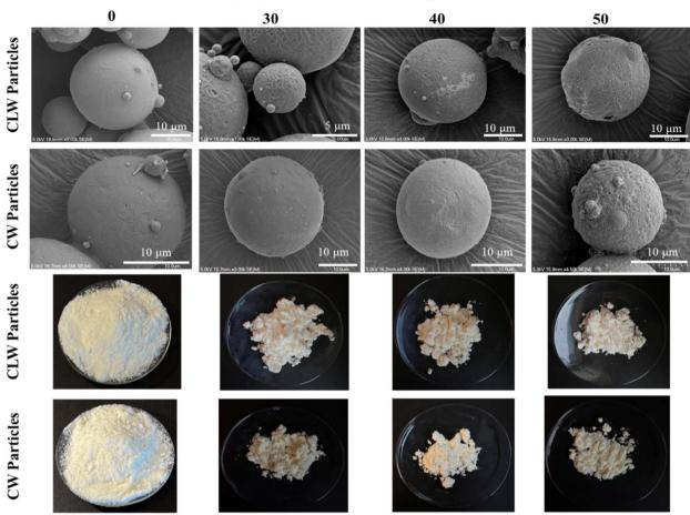
Fig. 2 SEM images (top) and the photographs (bottom) of the fish oil-loaded CLW and CW particles
