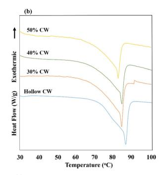
Fig. 5 Melting behavior of fish oil-loaded CLW particles (a) and CW particles (b)
