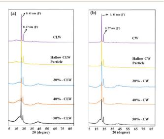
XRD patterns of fish oil-loaded CLW (a) and CW (b) particles
