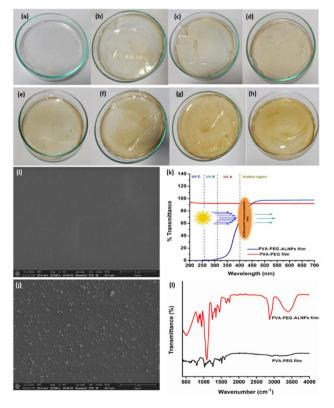
Fig. 3 PVA-PEG-A-LNPs-based packaging films containing (a) no ALNPs, and (b) 1%, (c) 3%, (d) 5%, (e) 7%, (f) 10%, (g) 15%, and (h) 20% BB@ALNPs, and characterization of packaging films: (i) SEM of a bare PVA-PEG film, (j) SEM of PVA-PEG\_BB@ALNPs, (k) UV blocking properties, and (I) FTIR spectrum of films.
