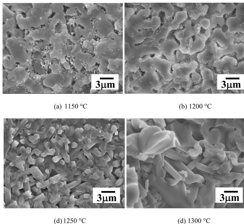
Fig. 9 SEM micrographs of the fracture surface of HA samples sintered at (a) 1150 °C, (b) 1200 °C, (c) 1250 °C and (d) 1300 °C.
