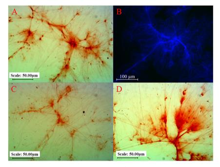
Fig. 3 Light microscopy images of rehydrated CSM at 20× magnification: (A) R, (C) H, and (D) M. (B) CLSM image of rehydrated R at 25× magnification.
