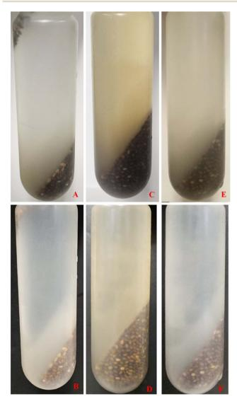
Fig. 1 CSM separation after the centrifugation process for R, H, and M against a white and black background. R: A and B; H: C and D; M: E and
