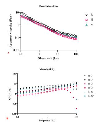
Fig. 8 (A) Apparent viscosity against shear rate curves and (B) viscoelastic properties of CSM.
