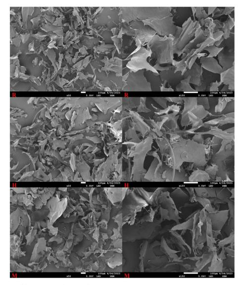
SEM micrographs of CSM powder at  $50 \times$  and  $150 \times$  magnifications
