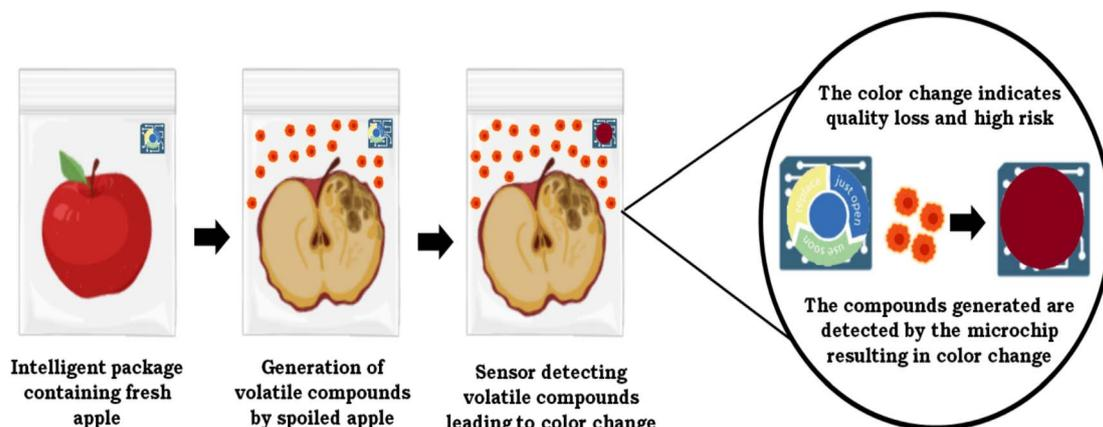
Fig. 3 Spoilage detection mechanism of indicators and sensors.
