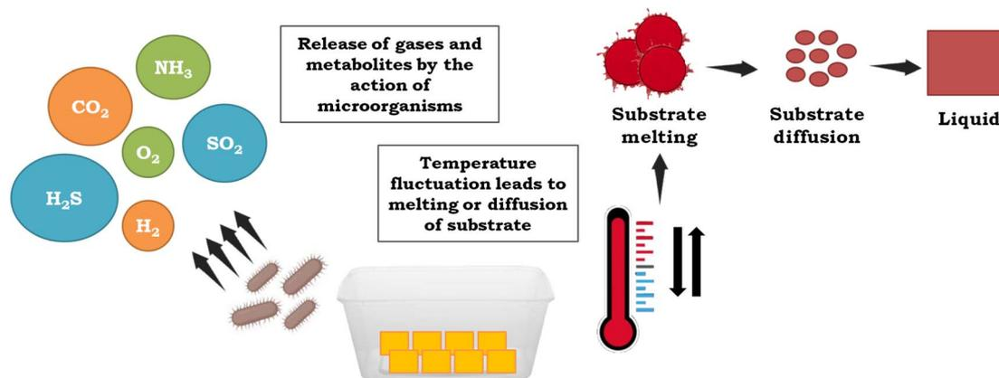
Fig. 4 Mechanism behind color-changing intelligent packaging systems.
