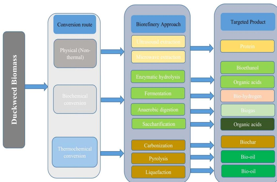
Fig. 4 . Duckweed biorefinery processes and integrated products.
