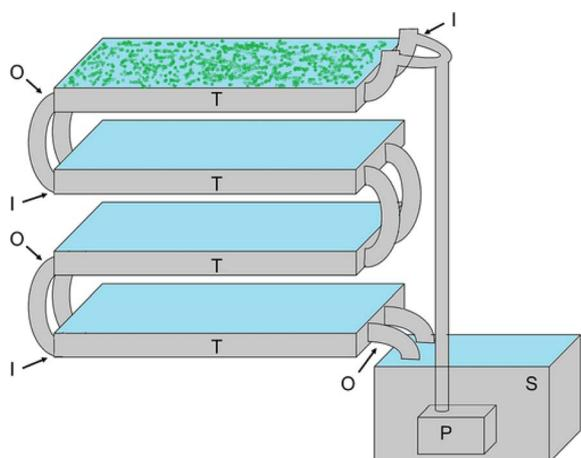
Fig. 1 Schematic overview of a multi-tiered duckweed bioreactor. S – sump; P – pump; t – duckweed trays; I – tray inlets; O – tray outlets.<sup>69</sup>
