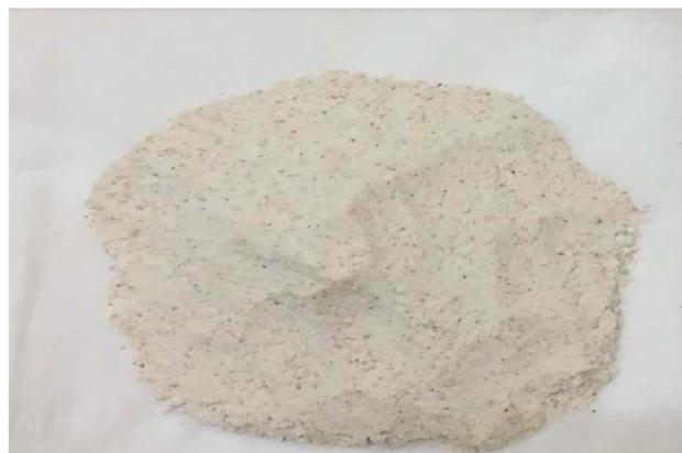
Fig. 1 BoxBadam Nano Cellulose Particles (BBNCPS) obtained after physico-chemical treatment.
