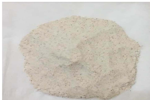
Fig. 1 BoxBadam Nano Cellulose Particles (BBNCPs) obtained after physio-chemical treatment.
