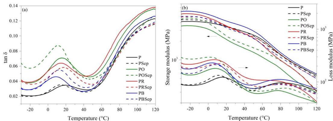
Fig. 5 (a)  $\tan \delta$  and (b) storage ( $E'$ ) and loss ( $E''$ ) modulus results for pure PHBV and PHBV compositions (solid lines: compositions without sepiolite; dashed lines: compositions with sepiolite).
