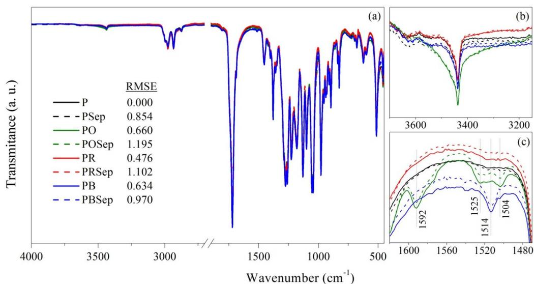
Fig. 2 (a) ATR-FTIR spectra of pure PHBV and PHBV compositions containing sepiolite (dashed lines) and different essential oils; (b) and (c) details of the main changes observed.
