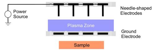
Scheme of a corona discharge plasma system with ground screen.
