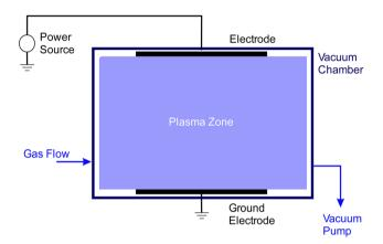
Fig. 2 Scheme of the glow discharge plasma system.
