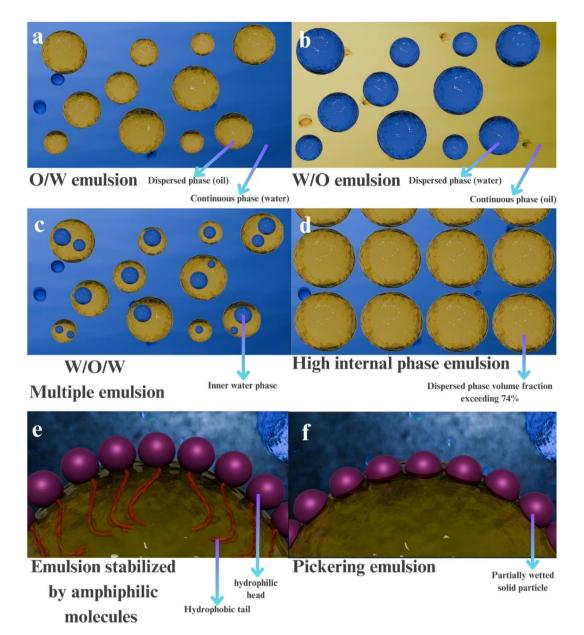
Fig. 1 Structural comparison of the main emulsion types ((a): oil in water emulsion; (b): water in oil emulsion; (c): water in oil in water emulsion; (d): high internal phase emulsion; (e): emulsion stabilized by amphiphilic molecules; (f): pickering emulsion). Created with Blender.
