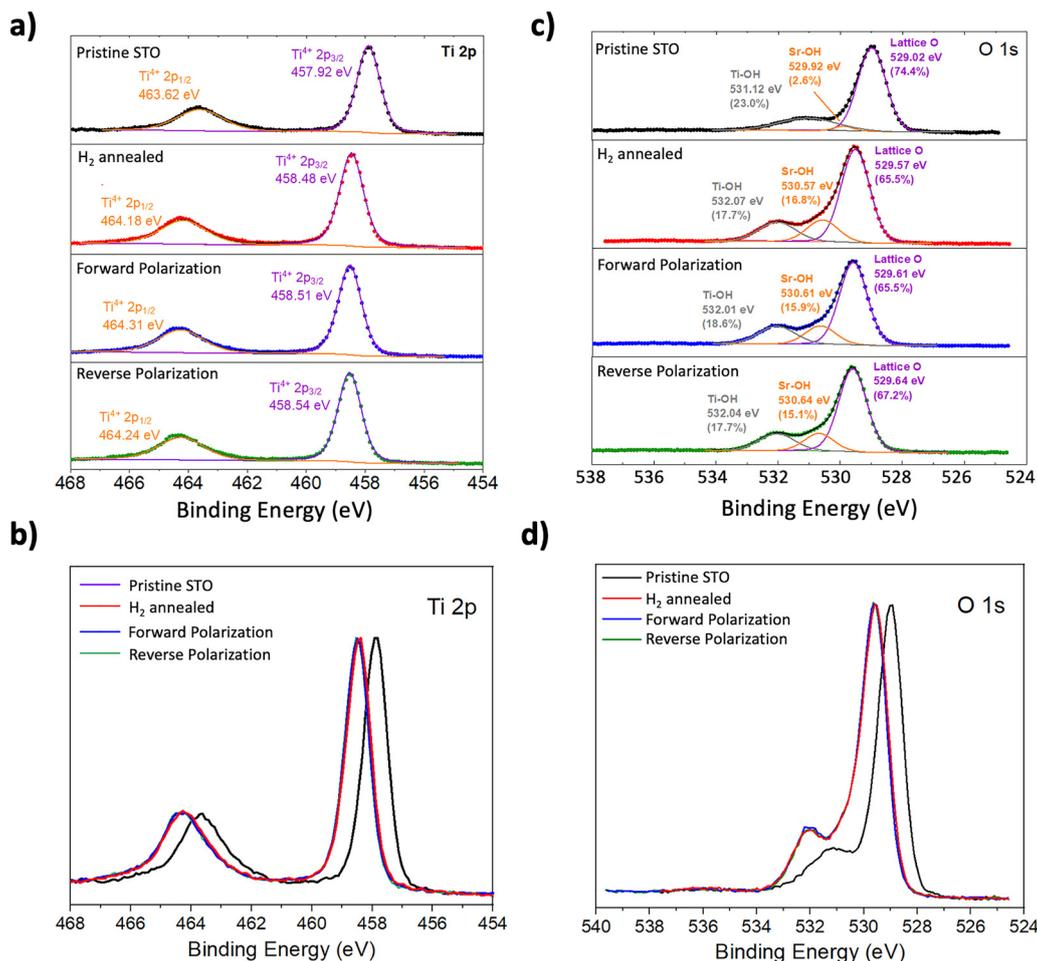
Fig. 6 (a) Peak fit and (b) overlap of the Ti 2p spectra of pristine SrTiO<sub>3</sub> (purple), H<sub>2</sub>-annealed SrTiO<sub>3-x</sub> without polarization (red), with forward polarization (blue) and reverse polarization (green), respectively. (c) Peak fit and (d) overlap of the O 1s spectra.
