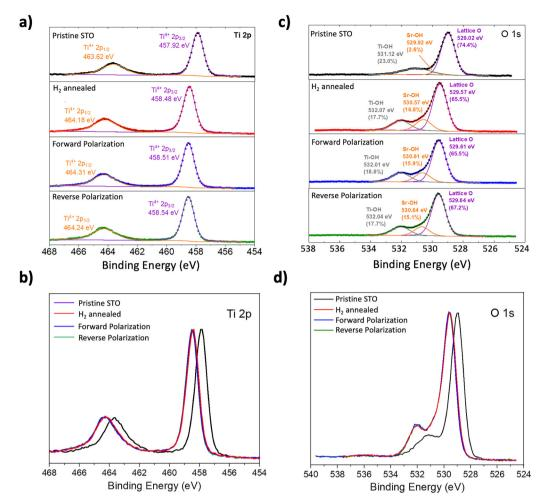
Fig. 6 (a) Peak fit and (b) overlap of the Ti 2p spectra of pristine  $SrTiO_3$  (purple),  $H_2$ -annealed  $SrTiO_{3-x}$  without polarization (red), with forward polarization (blue) and reverse polarization (green), respectively. (c) Peak fit and (d) overlap of the O 1s spectra.
