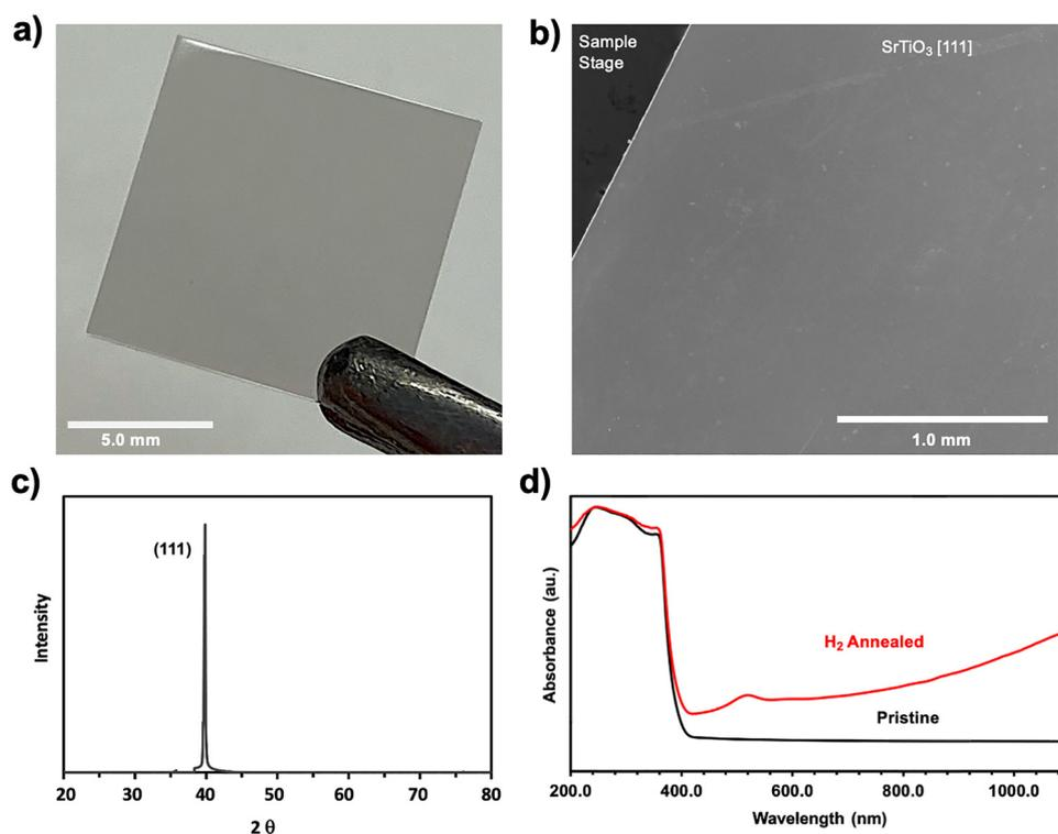
Fig. 2 (a) Photo of (111) SrTiO<sub>3</sub> single crystal, as purchased. (b) SEM image of SrTiO<sub>3</sub> single crystal surface after H<sub>2</sub> annealing. (c) XRD Pattern of H<sub>2</sub> annealed SrTiO<sub>3–x</sub> single crystal, confirming the (111) orientation (d) Optical absorbance spectra before and after H<sub>2</sub> annealing.
