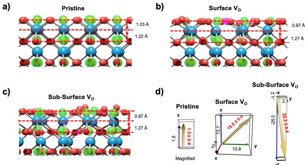
Fig. 7 Calculated structures for the pristine (111)  $\text{SrTiO}_3$  surface (a) before and after the introduction of a (b) surface oxygen vacancy (pink spheres) or a (c) sub-surface oxygen vacancy. Ti ions are shown as blue spheres and Sr ions as green spheres. (d) Calculated electric dipole density [ $\text{D}/\text{nm}^2$ ] is represented by arrows (pointing from negative to positive charge).
