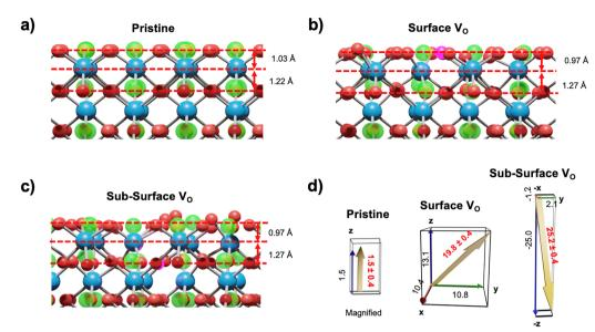
Fig. 7 Calculated structures for the pristine (111) SrTiO<sub>3</sub> surface (a) before and after the introduction of a (b) surface oxygen vacancy (pink spheres) or a (c) sub-surface oxygen vacancy. Ti ions are shown as blue spheres and Sr ions as green spheres. (d) Calculated electric dipole density [D/nm²] is represented by arrows (pointing from negative to positive charge).
