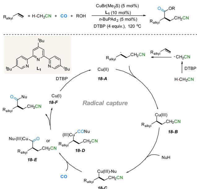
Fig. 18 Radical capture via radical cascade process.
