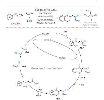
Fig. 14 Copper-catalyzed 1,2-dicarbonylative cyclization of alkenes *via* radical relav.
