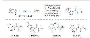
Fig. 25 Copper-catalyzed double carbonylation of indoles and alcohols
