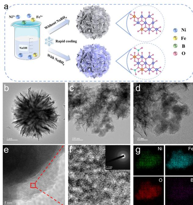
Fig. 1 Morphological characterization of a-B-NiFeO<sub>x</sub>H<sub>y</sub>. (a) Schematic diagram of the synthesis of a-B-NiFeO<sub>x</sub>H<sub>y</sub> and a-NiFeO<sub>x</sub>H<sub>y</sub>. (b)–(d) TEM, (e) and (f) high-resolution TEM (selected area electron diffraction), and (g) elemental mapping images of a-B-NiFeO<sub>x</sub>H<sub>y</sub>.
