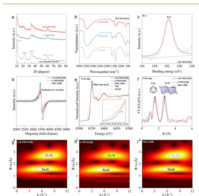
**Fig. 2** Structural characterization of a-B-NiFeO<sub>x</sub>H<sub>y</sub>. (a) XRD patterns. (b) FTIR spectra. (c) B 1s XPS of a-B-NiFeO<sub>x</sub>H<sub>y</sub>. (d) EPR spectra. (e) Ni K-edge of XANES spectra. (f) Ni K-edge of Fourier-transform EXAFS spectra. (g)–(i) The WT contour plots of a-B-NiFeO<sub>x</sub>H<sub>y</sub>, a-NiFeO<sub>x</sub>H<sub>y</sub> and NiFe LDH.
