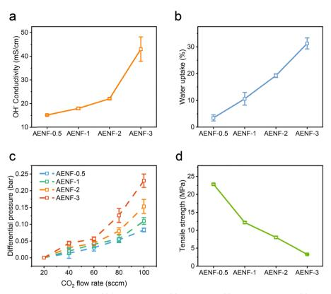
Fig. 3 Physico-chemical characterizations of AENF-x. (a) OH<sup>-</sup> conductivity, (b) water uptake, (c) gas permeability and (d) mechanical strength under the wetted state.
