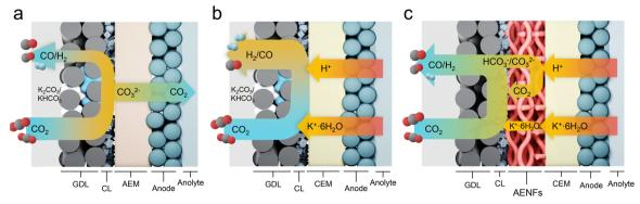
Scheme 1 Electrocatalytic  $CO_2$  reduction (e $CO_2R$ ) in zero-gap membrane electrode assemblies (MEAs). (a) Alkaline/neutral conditions with AEM, (b) acidic conditions with CEM, and (c) acidic conditions with the bipolar AENFs/CEM proposed in this study.
