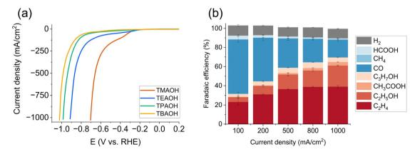
Fig. 1 (a) Linear-sweep voltammograms recorded in different tetraalkylammonium hydroxide solutions (1.0 M) under  $CO_2$  gas. (b) Faradaic efficiency of  $CO_2$ RR in 1.0 M tetramethylammonium hydroxide solutions at different current densities.
