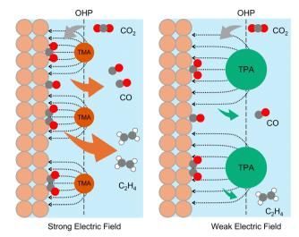
Fig. 4 Schematic of effect of different tetraalkylammonium cations on CO<sub>2</sub>RR
