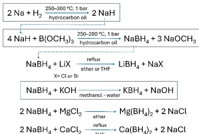
Scheme 2 Synthesis of tetrahydroborates (industrial processes are indicated by boxes).<sup>149,211–215</sup>
