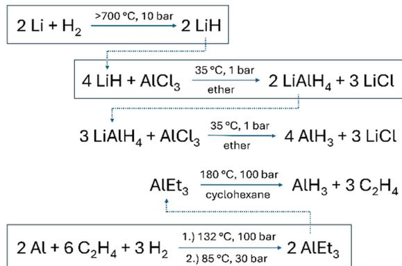
Scheme 1 Synthesis of  $\text{AlH}_3$  and LiH (industrial processes are indicated by the boxes).<sup>149–153</sup>
