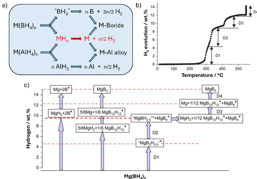
Fig. 3 (a) Simplified decomposition scheme for metal hydrides, tetrahydroborates, and tetrahydroaluminates, (b) volumetric temperature programmed desorption curve of  $\text{Mg}(\text{BH}_4)_2$  and (c) decomposition pathways of  $\text{Mg}(\text{BH}_4)_2$  (observed hydrogen evolution steps, see panel (b), marked by dashed lines; amorphous phases denoted by asterisks). Reproduced from ref. 72 with permission from Elsevier Ltd, copyright 2008.
