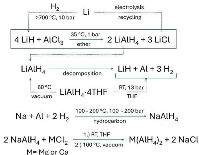
Scheme 3 Synthesis of tetrahydroaluminates (industrial processes are indicated by a box, RT = room temperature).<sup>149,217,242,258</sup>
