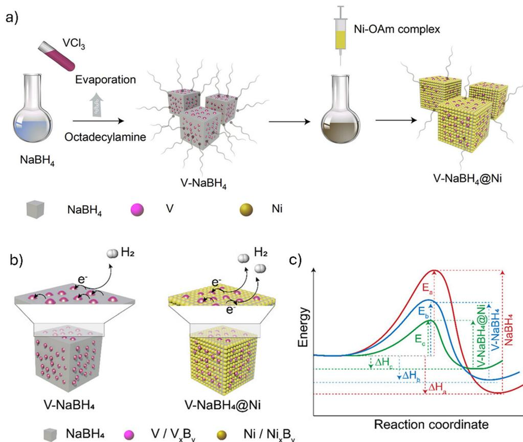
Fig. 5 (a) Illustration of the synthesis of vanadium-doped cube-like NaBH<sub>4</sub> with nickel shells, (b) the hydrogen release via the electron transfer process, and (c) the energy diagram showing altered thermodynamics and kinetics compared to pristine NaBH<sub>4</sub>. Reproduced from ref. 198 with permission from the American Chemical Society, copyright 2023.
