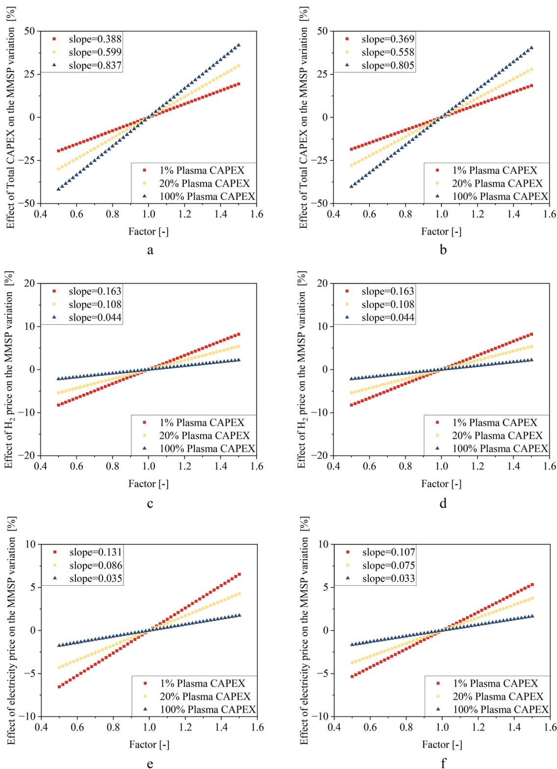
Fig. 10 One-factor sensitivity analysis, at different plasma CAPEX. Showing the effect of increasing and decreasing total CAPEX at the fractional methanol yields (a)  $Y = 0.11$  and (b)  $Y = 0.23$ ,  $H_2$  price at (c)  $Y = 0.11$  and (d)  $Y = 0.23$ , and surplus electricity price at (e)  $Y = 0.11$  and (f)  $Y = 0.23$  between 0.5 and 1.5 times the original value.
