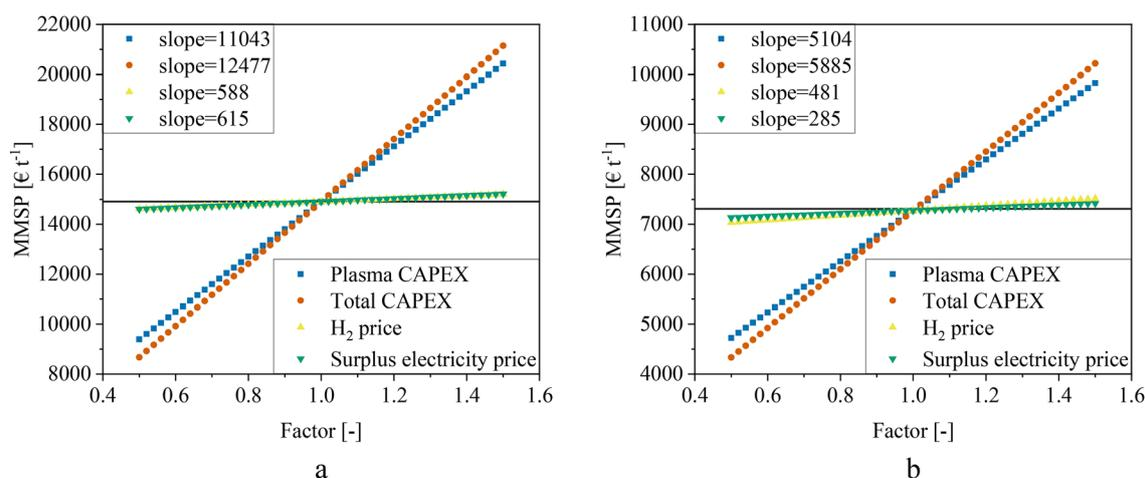
Fig. 7 One-factor sensitivity analysis showing the effect of increasing and decreasing plasma CAPEX, total fixed cost, H<sub>2</sub> price, and surplus electricity price between 0.5 and 1.5 times the original value for the two fractional methanol yields (a)  $Y = 0.11$  and (b)  $Y = 0.23$ .
