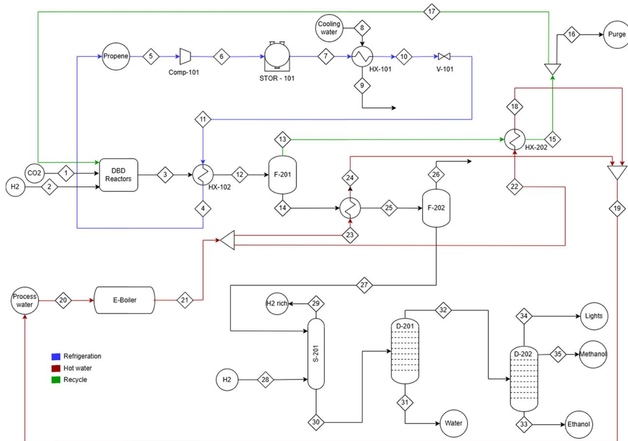
Fig. 1 PFD showing a fully continuous system.
