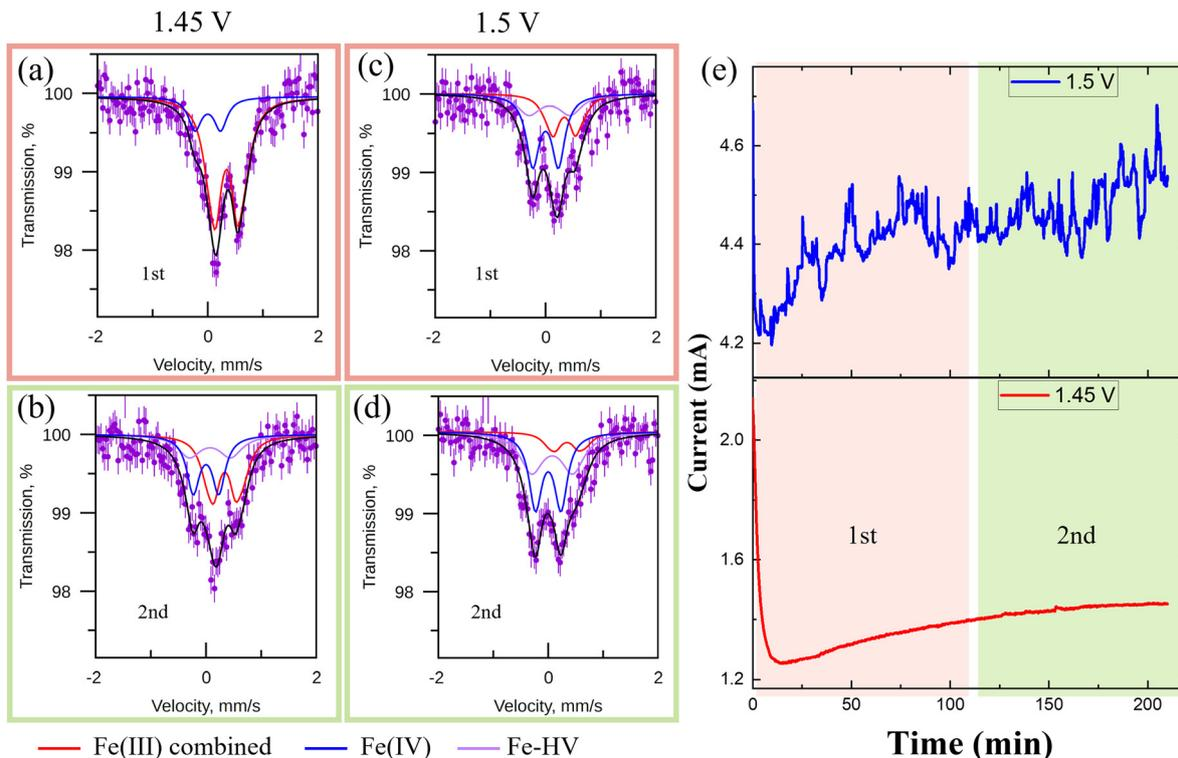
**Fig. 3** The transition from Fe(III) to tetravalent Fe near the OER onset potential: (a) and (b) and (c) and (d) Mössbauer spectra from the 1st and 2nd half of the 3.5 h potential holds at 1.45 V and 1.5 V, respectively. Fe species colored as in Fig. 2. (e) Chronopotentiometry at potentials near the OER onset.
