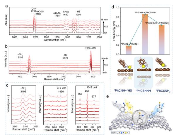
Fig. 5 (a) Quasi-in situ IR and (b and c) Quasi-in situ Raman spectra of PhCN hydrogenation to PhCSNH<sub>2</sub> in the presence of N-GC-6 recorded within 3500–600 cm<sup>-1</sup> by flowing H<sub>2</sub>S (5 wt%) as a reaction gas; (d) free energy diagram for the \*PhCNH, \*PhCSHNH and \*PhCSNH<sub>2</sub> formation process on pyridinic N; and (e) catalytic reaction mechanism of H<sub>2</sub>S nucleophilic addition of PhCN to PhCSNH<sub>2</sub> over N-GC-6.
