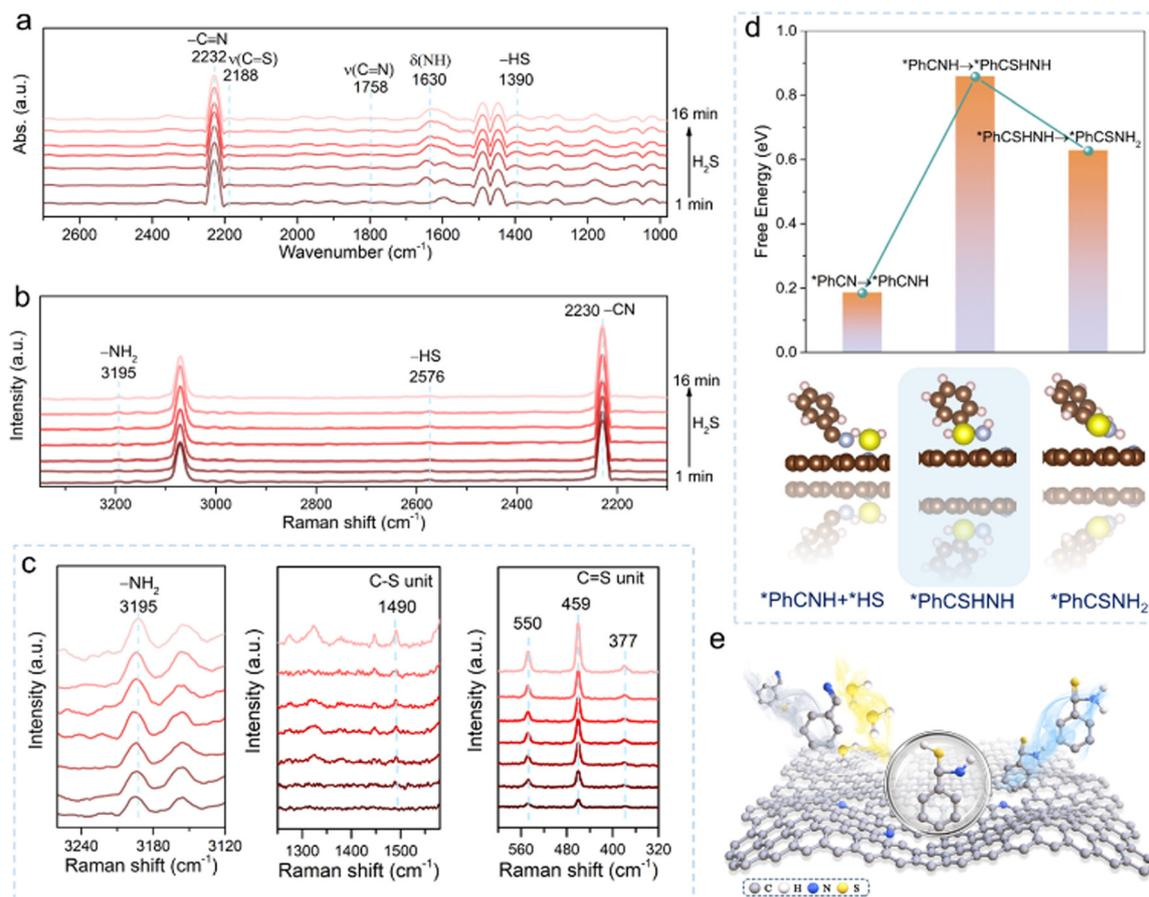
Fig. 5 (a) Quasi-*in situ* IR and (b and c) Quasi-*in situ* Raman spectra of PhCN hydrogenation to PhCSNH<sub>2</sub> in the presence of N-GC-6 recorded within 3500–600 cm<sup>-1</sup> by flowing H<sub>2</sub>S (5 wt%) as a reaction gas; (d) free energy diagram for the \*PhCNH, \*PhCSNHNH and \*PhCSNH<sub>2</sub> formation process on pyridinic N; and (e) catalytic reaction mechanism of H<sub>2</sub>S nucleophilic addition of PhCN to PhCSNH<sub>2</sub> over N-GC-6.
