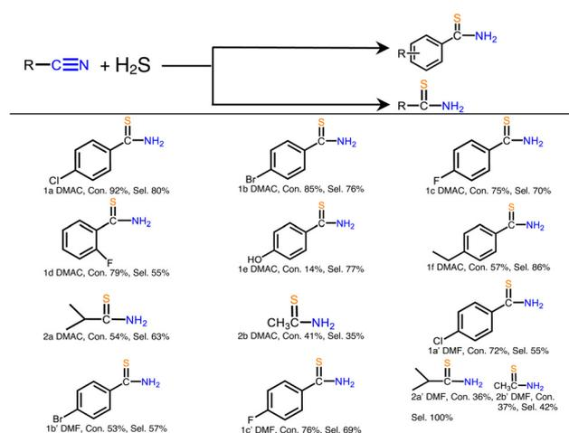
Reaction conditions: 4 mmol nitriles in 40 mL of solvents (DMAC and DMF) using 40 mg of a catalyst, reaction for 2 h at 60 °C under atmospheric pressure H<sub>2</sub>S (5 wt%, 20 mL min<sup>-1</sup>).
