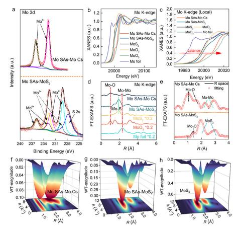
Fig. 3 Local structural evolution of Mo SAs-Mo Cs into Mo SAs-MoS<sub>2</sub> catalysts. (a) XPS spectra, Mo K-edge in (b) XANES and (c) adsorption edge, (d) EXAFS and (e) EXAFS fitting curves. WT contour plots of (f) Mo SAs-Mo Cs, (g) Mo SAs-MoS<sub>2</sub>, and (h) MoS<sub>2</sub>:
