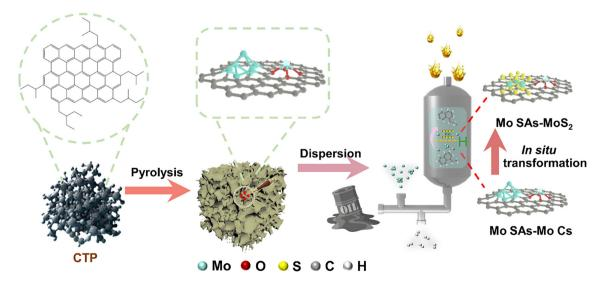
Fig. 1 Schematic of the catalyst preparation process
