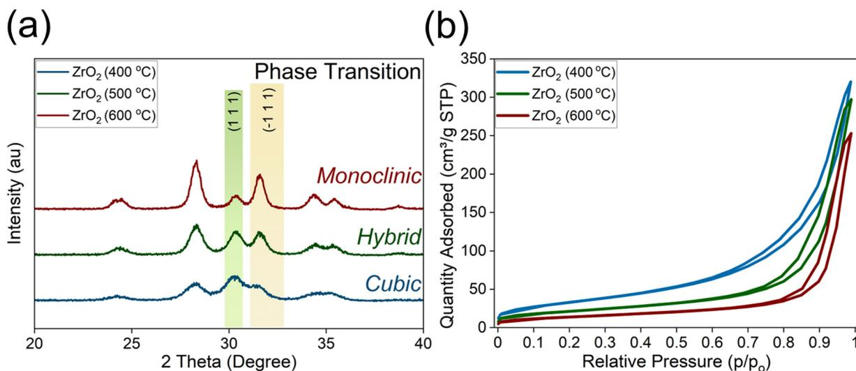
Fig. 1 (a) XRD revealing the effect of calcination temperature on ZrO<sub>2</sub> phases; (b) Nitrogen isotherms at different temperatures on different zirconia calcination temperatures.
