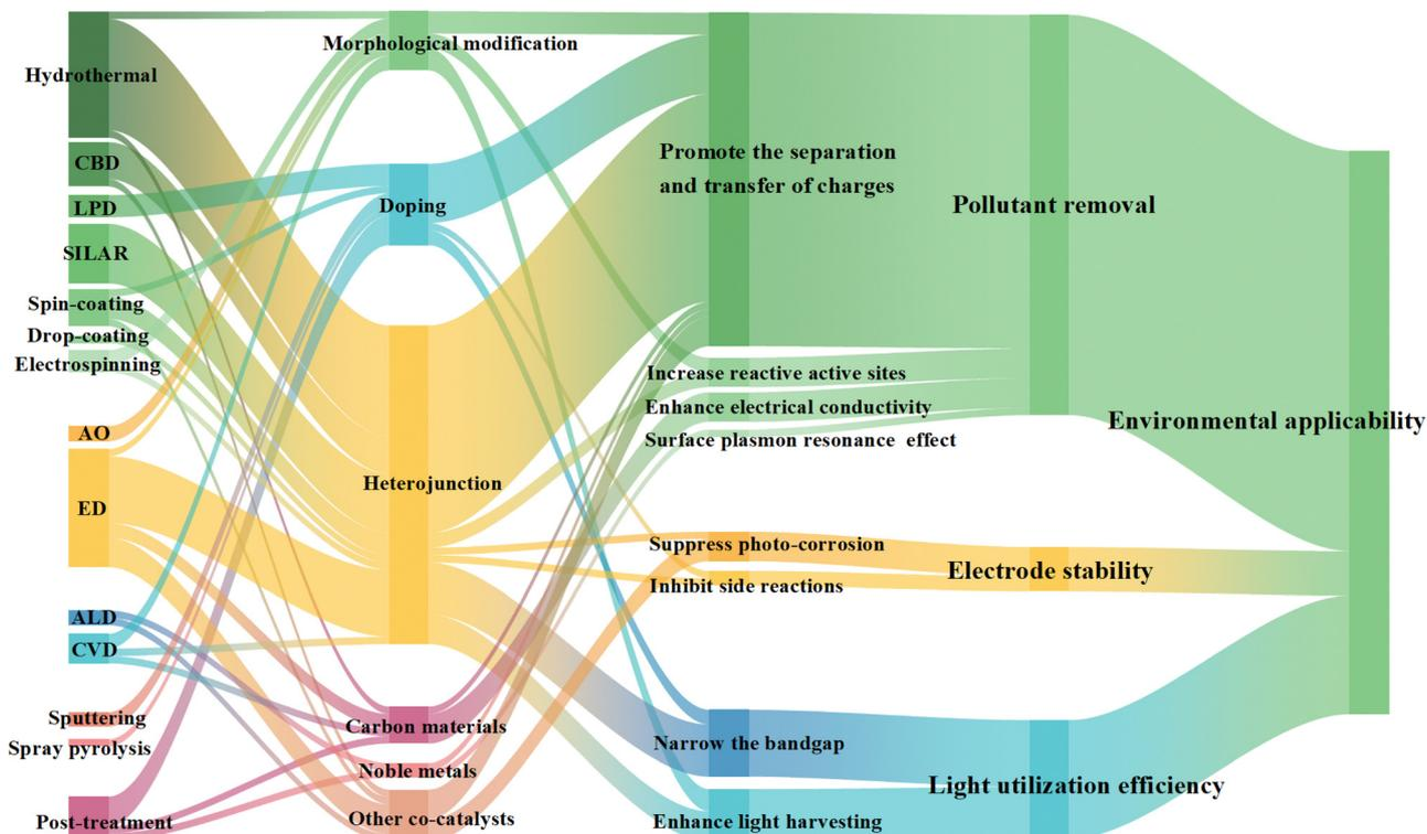
Fig. 5 The synthesis–structure–mechanism–activity relationship diagram of non-TiO<sub>2</sub>-based photoanodes based on literature statistics. (The results of the Sankey diagram are derived from 76 pieces of literature on non-TiO<sub>2</sub>-based photoanodes for pollutant wastewater treatment.)
