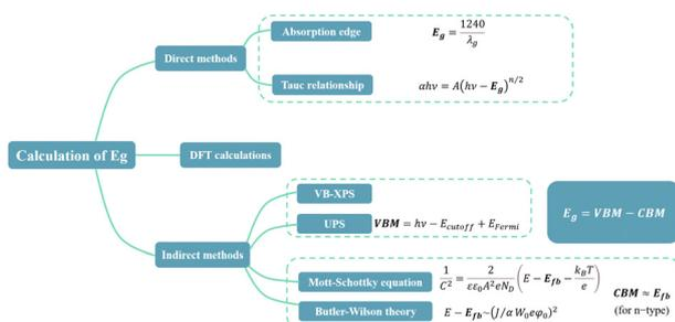
Fig. 6 Methods for the determination of  $E_g$ .
