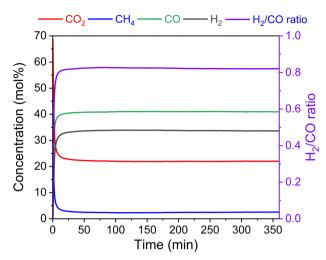
Fig. 8 Performance of the post-plasma-catalytic DRM reaction using 4NiAl-act sample. Real-time reactant and product concentrations and syngas ratio for 30 vol%  $CH_4$  fraction at the inlet for 6 h. The 4NiAl sample was ex situ activated  $(H_2/N_2 = 1/1, T = 750 \, ^{\circ}C)$  prior to testing.
