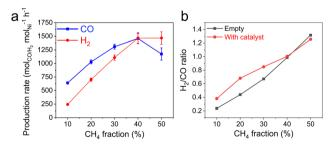
Fig. 6 Performance of the post-plasma-catalytic DRM reaction using 4NiAl-act sample. (a) Molar production rate of CO and  $H_2$  in relation to Ni loading, and (b) syngas ratio ( $H_2/CO$ ) as a function of increasing CH<sub>4</sub> inlet concentration. The 4NiAl sample was *ex situ* activated ( $H_2/N_2 = 1/1$ , T = 750 °C) prior to testing.
