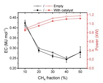
Fig. 7 Performance of the post-plasma-catalytic DRM reaction using 4NiAl-act sample. Energy cost (per mol of reactant mixture) for total conversion as a function of increasing inlet CH<sub>4</sub> fraction. The 4NiAl sample was ex situ activated ( $H_2/N_2 = 1/1$ , T = 750 °C) prior to testing
