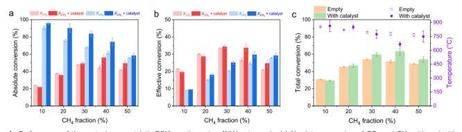
Fig. 4 Performance of the post-plasma-catalytic DRM reaction using 4NiAl-act sample. (a) Absolute conversion of  $CO_2$  and  $CH_4$  with and without catalyst, (b) effective conversion of  $CO_2$  and  $CH_4$  with and without catalyst, and (c) total conversion of  $CO_2$  and  $CH_4$  with and without catalyst. The 4NiAl sample was *ex situ* activated ( $H_2/N_2 = 1/1$ , T = 750 °C) prior to testing.
