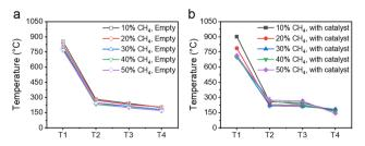
Fig. 5 Average temperature with (a) empty catalyst and (b) filled catalyst bed with 4NiAl. Recorded at four locations along reactor body (T1 = 1) inside catalyst bed, T2 = 10 cm from reactor outlet, T3 = 20 cm from reactor outlet, T4 = 30 cm from reactor outlet).
