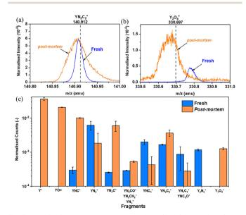
Fig. 5 ToF-SIMS Y-based fragments before (fresh) and after (postmortem) electrochemical testing of CNGO-0.50 Y in positive SIMS spectrum shown for (a)  $YN_2C_2^+$ , (b)  $Y_3O_4^+$ , and (c) list of identified major fragments. Fragment counts from peak areas were normalized to the total
