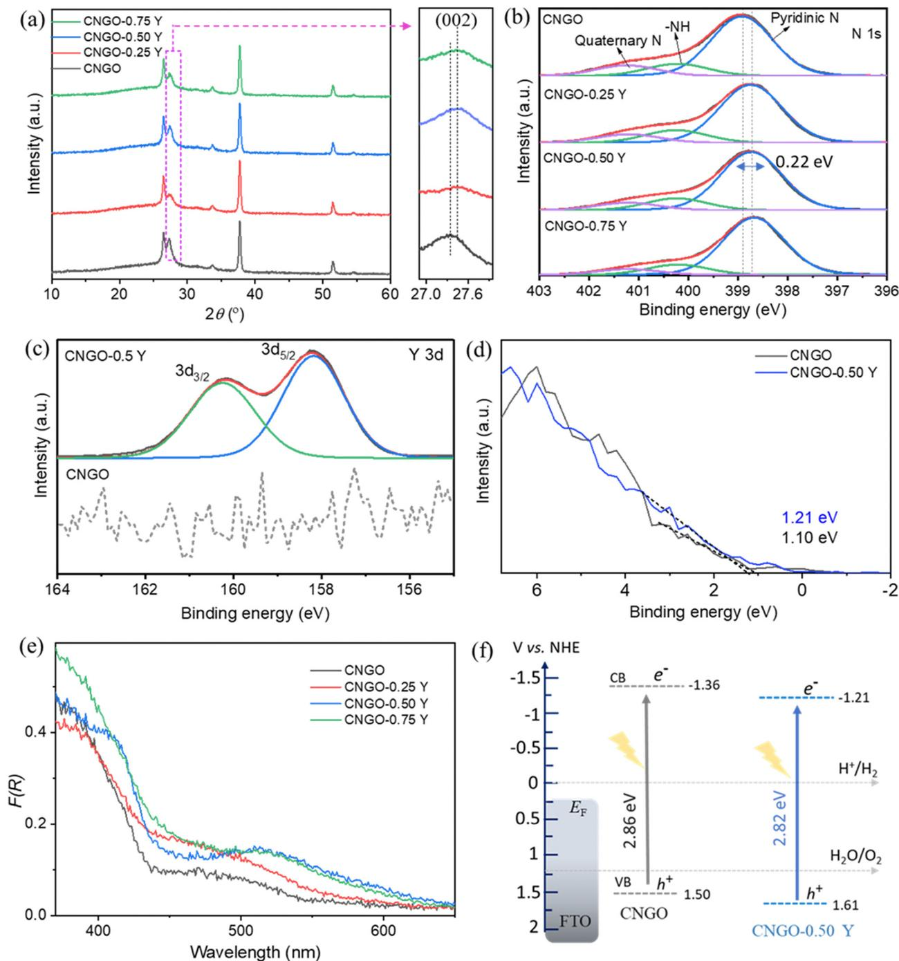
**Fig. 1** Characterization of CNGO and Y-cluster-modified CNGO films. (a) XRD. High-resolution XPS analysis: (b) N 1s, (c) Y 3d, (d) Valence band (VB) XPS (CNGO and CNGO-0.50 Y). (e) UV-vis DRS. (f) Schematic representation of the electronic band structure of CNGO and CNGO-0.50 Y films (on the normal hydrogen electrode (NHE) scale), determined using the VB position obtained from XPS measurement and the optical  $E_g$  calculation.
