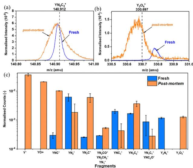
Fig. 5 ToF-SIMS Y-based fragments before (fresh) and after (*post-mortem*) electrochemical testing of CNGO-0.50 Y in positive SIMS spectrum shown for (a)  $YN_2C_2^+$ , (b)  $Y_3O_4^+$ , and (c) list of identified major fragments. Fragment counts from peak areas were normalized to the total ion counts.
