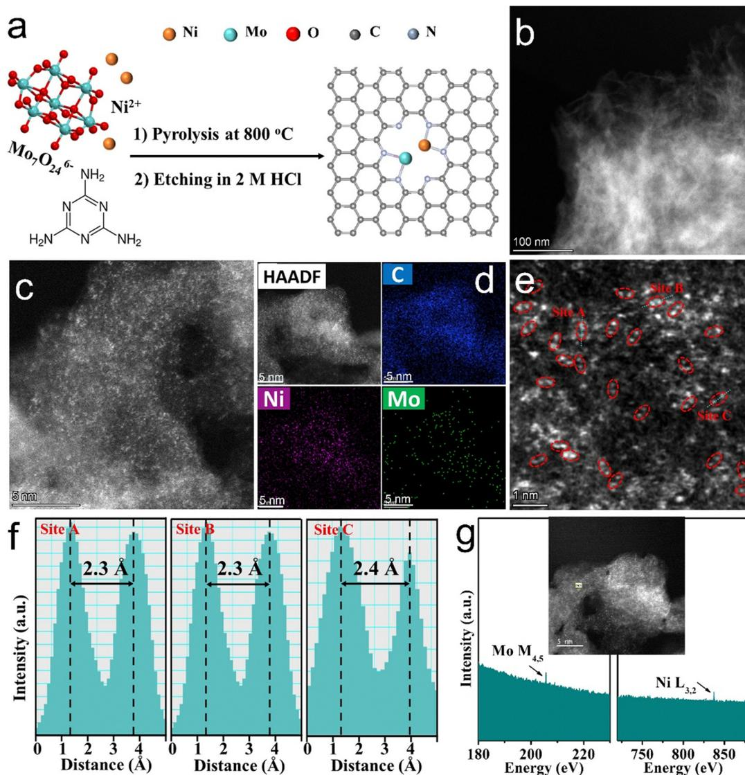
**Fig. 1** (a) Schematic of catalyst preparation; (b) and (c) HAADF-STEM image of NiMo-DASC; (d) EDX elemental mapping images of Ni, Mo and C in NiMo-DASC; (e) HAADF-STEM image of NiMo-DASC in which diatomic NiMo sites separated by a distance of 2.3 Å are highlighted with red circles for clarity; (f) intensity profiles for three diatomic sites of image (e); (g) EELS spectrum of NiMo atomic sites indicated in the inset with a white line.
