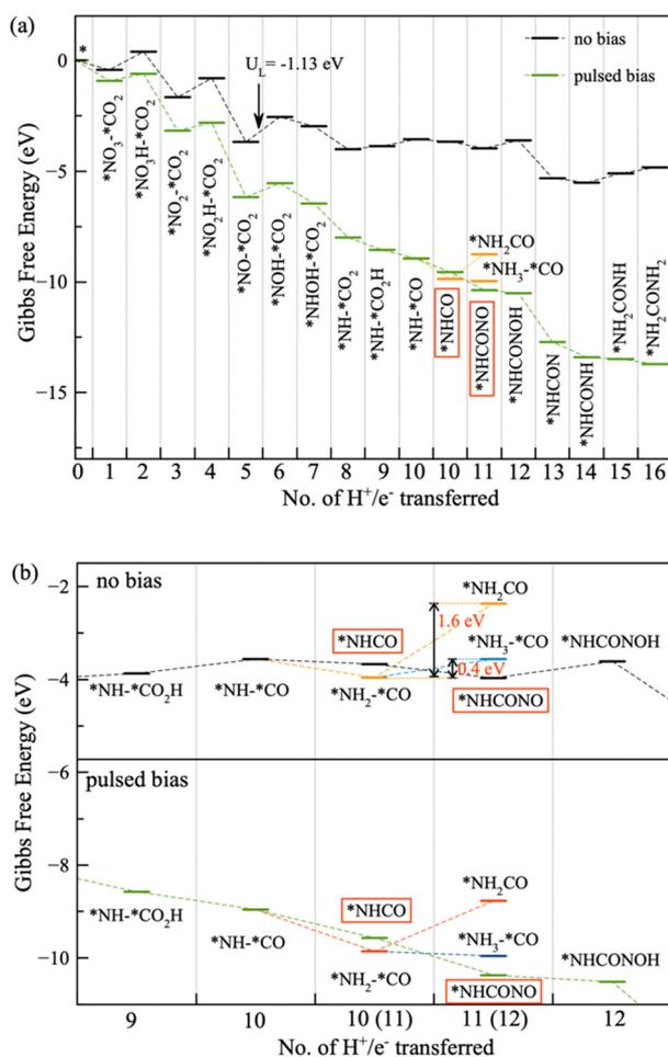
**Fig. 6** (a) Gibbs free energy reaction pathway for the urea formation. The hyphen indicates the adsorption of both species on different metals. The two C–N coupling steps are highlighted. (b) Competitive ammonia reduction path.
