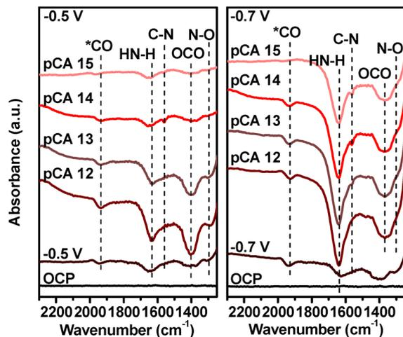
Fig. 4 *In situ* ATR-SEIRAS spectra recorded for NiMo-DASC at two different potentials under pulsed conditions.
