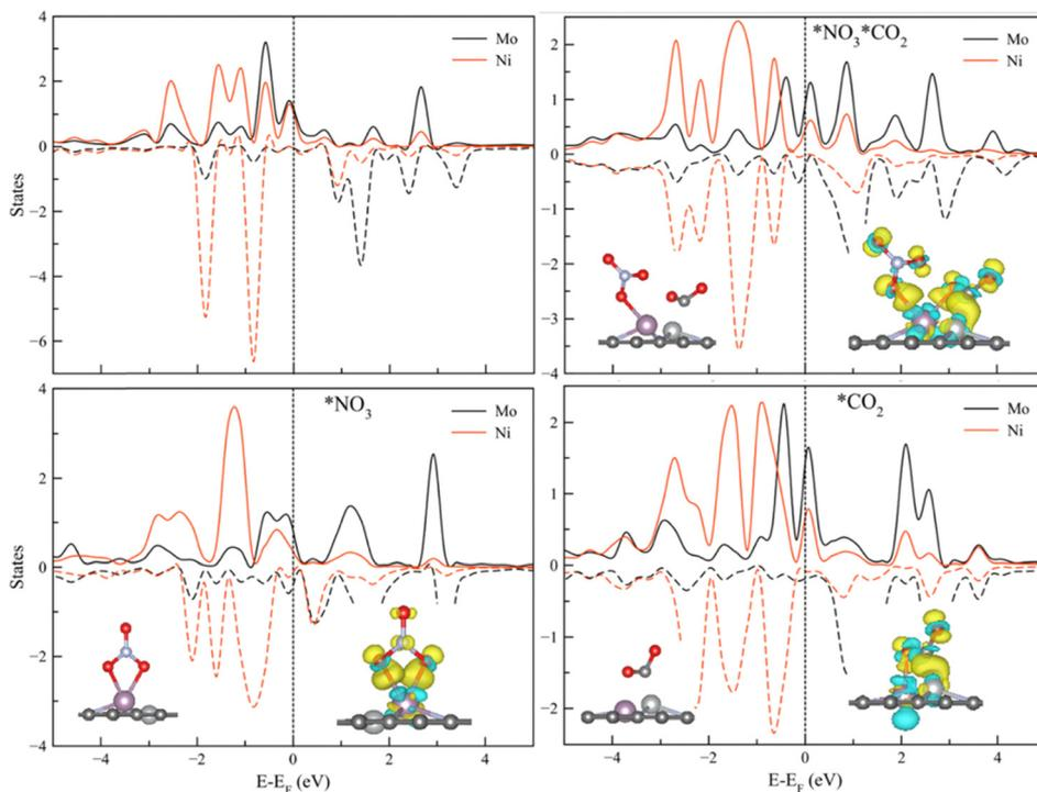
Fig. 5 Projected density of state (PDOS) analysis of the spin polarized d orbitals for the bare surface and the adsorption of the  $\text{NO}_3^-$  and  $\text{CO}_2$  gases (spin up in solid line, spin down with dotted line). The inset shows the charge density difference for the adsorption of  $\text{NO}_3^-$ ,  $\text{CO}_2$  and when adsorbed at the same time. The yellow (blue) color represents loss (accumulation) of electrons. The black dotted lines represent the Fermi energy level.
