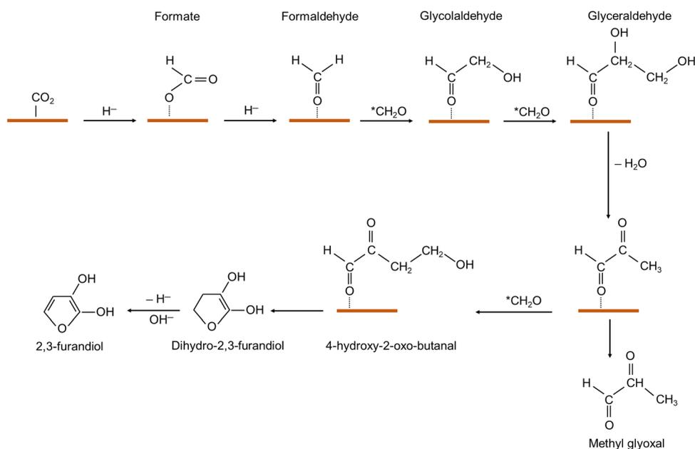
Fig. 1 Proposed mechanism for methyl glyoxal and 2,3-furandiol formation catalyzed by nickel phosphides.<sup>40</sup>
