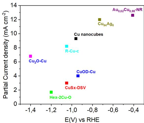
Fig. 4 Catalysts for CO<sub>2</sub>R to propanol in H-cells; partial current density as a function of applied cathode cell voltage. Data are given in Table 4.
