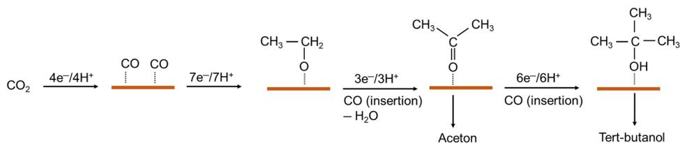
Fig. 7 Proposed mechanism for the formation of *tert*-butanol catalyzed by Cu<sub>0.48</sub>Ir<sub>0.52</sub> alloy.<sup>139</sup>
