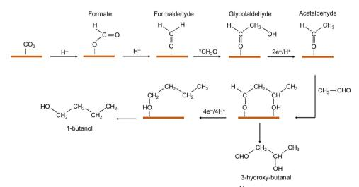
Fig. 2 Proposed mechanism for 1-butanol formation catalyzed by Ni-doped (Cr<sub>2</sub>O<sub>3</sub>)<sub>3</sub>Ga<sub>2</sub>O<sub>3</sub>.<sup>44</sup>
