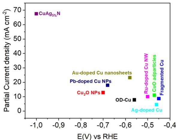
Fig. 5 Catalysts for COR to propanol in flow cells; partial current density as a function of applied cathode cell voltage. Data are given in Table 5.
