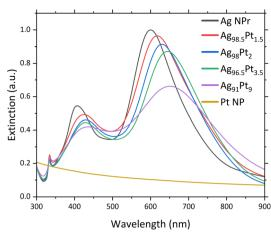
Fig. 1 UV-vis spectra of AgPt surface alloyed catalyst with different Pt loading
