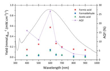
Fig. 7 Wavelength-dependent product yields normalised by laser power. Black line shows extinction spectra for Ag<sub>91</sub>Pt<sub>9</sub> post-reaction.
