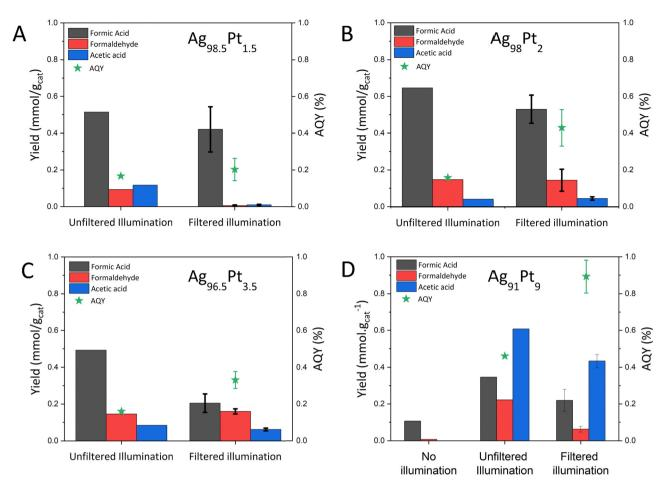
Fig. 5 Product yields and AQY under unfiltered Xe lamp illumination (320–2500 nm) and Filtered Xe lamp illumination (380–780 nm) of (A) Ag<sub>98.5</sub>Pt<sub>1.5</sub> (B)  $Ag_{98}Pt_2$  (C)  $Ag_{95.5}Pt_{3.5}$  (D)  $Ag_{91}Pt_9$  reaction conditions  $-\sim 10$  mg catalyst, P=10 bar,  $H_2/CO_2$  (1:1 v/v), t=2 h.
