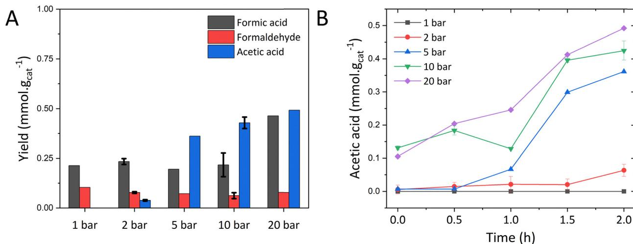
Fig. 6 (A) Product yield of Ag<sub>91</sub>Pt<sub>9</sub> as a function of pressure (B) CH<sub>3</sub>COOH yield profile at different pressures. Reaction conditions – ~10 mg catalyst, H<sub>2</sub>/CO<sub>2</sub> (1 : 1), room temperature, filtered illumination mode.
