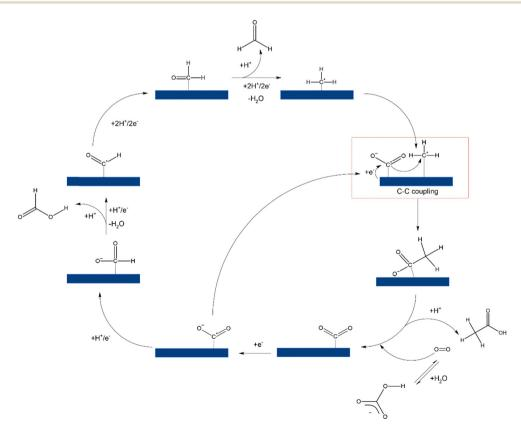
Scheme 1 Proposed reaction pathway of CO<sub>2</sub> to HCOOH, HCHO and CH<sub>3</sub>COOH on AgPt NPr.
