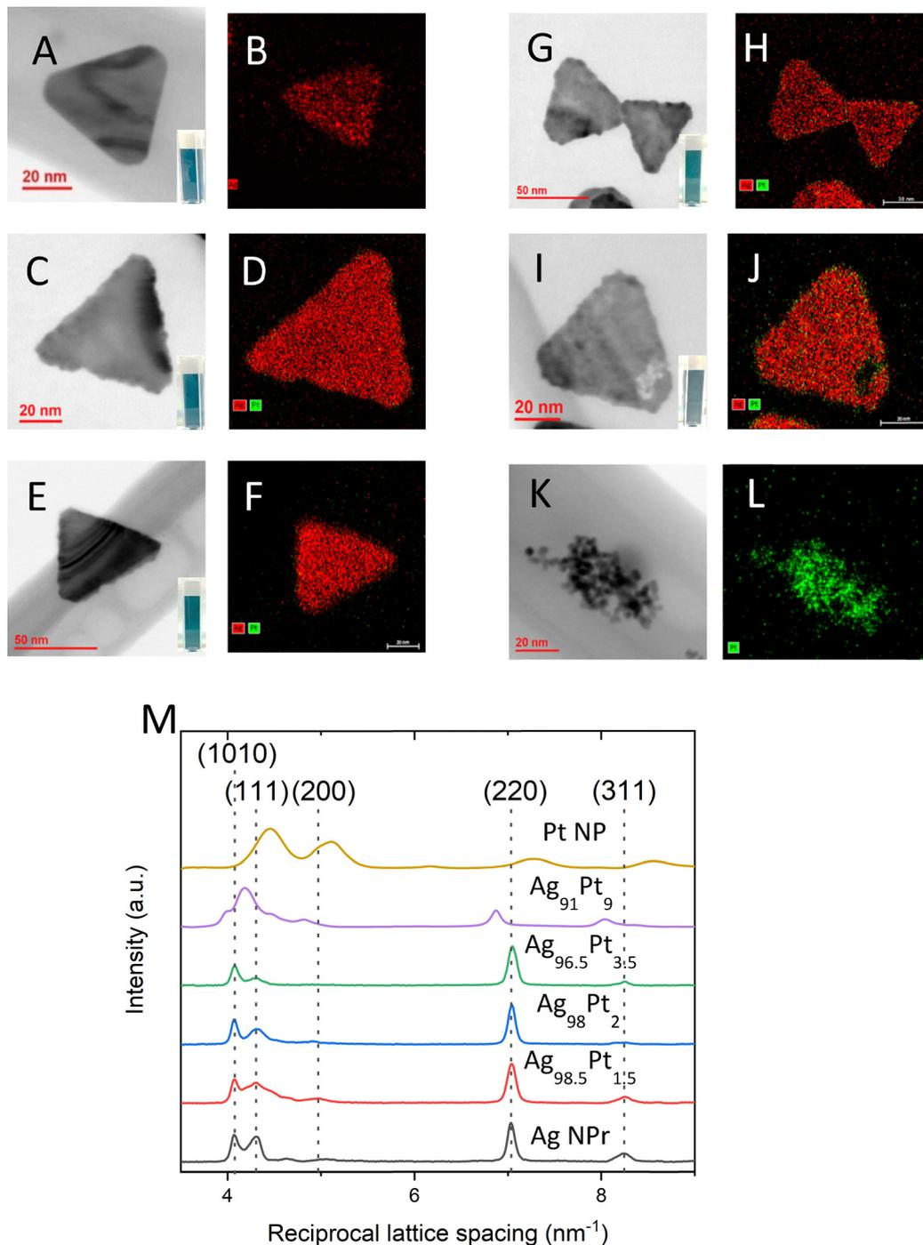
Fig. 2 (A)–(L) STEM-EDS micrographs of (A) and (B) Ag NPr (C) and (D)  $\text{Ag}_{98.5}\text{Pt}_{1.5}$  (E) and (F)  $\text{Ag}_{98}\text{Pt}_2$  (G) and (H)  $\text{Ag}_{96.5}\text{Pt}_{3.5}$  (I) and (J)  $\text{Ag}_{91}\text{Pt}_9$  (K) and (L) Pt NP (inset of STEM micrographs shows corresponding bulk sample solutions) with corresponding elemental maps of Ag (red) and Pt (green) (M) rotational averages of selected area diffraction (SAED) patterns of corresponding catalysts.
