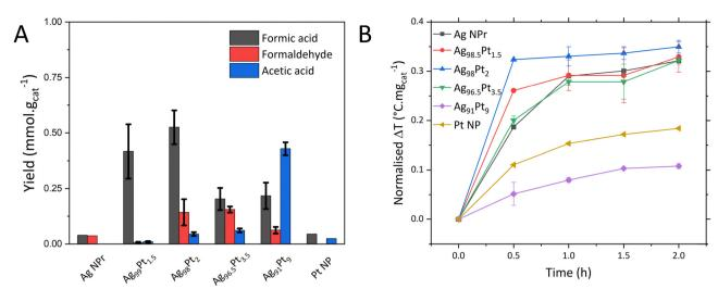
Fig. 4 (A) Product yield of AgPt surface alloyed catalysts with different Pt loadings (B) in situ temperature profile of the reactor solution. Reaction conditions – pressure = 10 bar ( $H_2/CO_2 = 1$ ), filtered Xe lamp illumination, t = 2 h.
