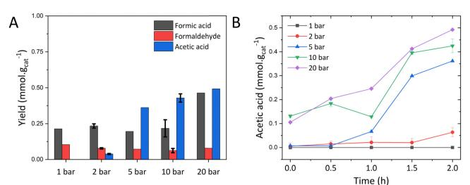
Fig. 6 (A) Product yield of  $Ag_{91}Pt_9$  as a function of pressure (B)  $CH_3COOH$  yield profile at different pressures. Reaction conditions  $-\sim 10$  mg catalyst, H<sub>2</sub>/CO<sub>2</sub> (1:1), room temperature, filtered illumination mode.
