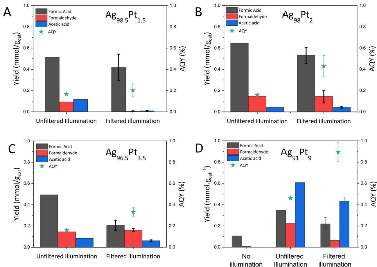
Fig. 5 Product yields and AQY under unfiltered Xe lamp illumination (320–2500 nm) and Filtered Xe lamp illumination (380–780 nm) of (A) Ag<sub>98.5</sub>Pt<sub>1.5</sub> (B) Ag<sub>98</sub>Pt<sub>2</sub> (C) Ag<sub>96.5</sub>Pt<sub>3.5</sub> (D) Ag<sub>91</sub>Pt<sub>9</sub> reaction conditions – ~10 mg catalyst,  $P = 10$  bar, H<sub>2</sub>/CO<sub>2</sub> (1:1 v/v),  $t = 2$  h.
