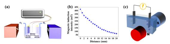
Fig. 6 (a) The illustration of electrolysis of water for oxygen evolution assisted by an external magnetic field; (b) the magnetic induction intensity *versus* magnet distance function curve; (c) the reference of parallel direction.
