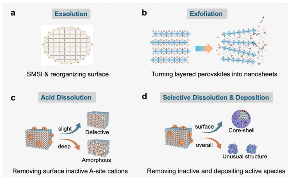
Fig. 3 Schematic illustration of chemical strategies for disassembling and reassembling perovskites. (a) The exsolution approach. (b) The exfoliation approach. (c) The acid dissolution approach. (d) The selective dissolution and deposition approaches. SMSI: strong metal–support interaction.
