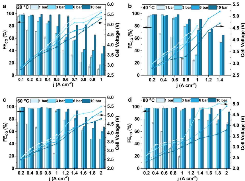
Fig. 1  $FE_{CO}$  and cell voltage as a function of current density for the  $CO_2RR$  at various pressures (1 bar, 3 bar, 6 bar, and 10 bar) and temperatures: (a) 20 °C, (b) 40 °C, (c) 60 °C, and (d) 80 °C. A consistent input flow of 250 sccm  $CO_2$  was employed in all experiments. The cathode was Ag GDE and the anode was Ir/Ti felt. 0.1 M  $KHCO_3$  was used as an anolyte. The error bars represent standard deviations of three independent measurements.
