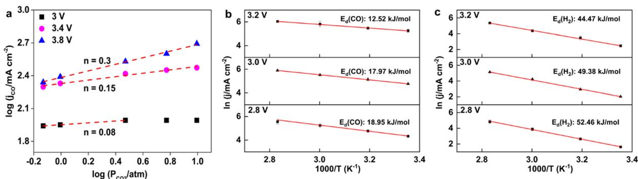
Fig. 3 (a) Reaction order for CO<sub>2</sub> derived from the logarithmic dependence of  $j_{\text{CO}}$  on CO<sub>2</sub> pressure at various applied cell voltages (3 V, 3.4 V, and 3.8 V) from a pressure range of 0.75 bar to 10 bar. (b)  $E_{\text{d}}$  for the CO<sub>2</sub>RR to CO at 2.8 V, 3 V, and 3.2 V at 1 bar. (c)  $E_{\text{d}}$  for the HER at 2.8 V, 3 V, and 3.2 V at 1 bar. The error bars represent the standard deviations of three independent measurements.
