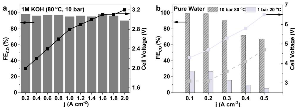
Fig. 5 (a) FE<sub>CO</sub> and cell voltage as a function of current density for the CO<sub>2</sub>RR in 1 M KOH anolyte at 80 °C and 10 bar. (b) Comparison of FE<sub>CO</sub> and cell voltage at varying current densities for the pure-water-fed CO<sub>2</sub>RR at 10 bar and 80 °C versus ambient conditions (1 bar, 20 °C).
