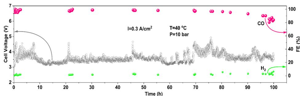
Fig. 4 Long-term stability test of the pressurized  $\text{CO}_2$  electrolyzer using a Ag cathode at 40 °C and 10 bar with a constant current density of 300  $\text{mA cm}^{-2}$ . The cell voltage (left axis, grey) and  $\text{FE}_{\text{CO}}$  (pink) and  $\text{H}_2$  (green) (right axis) are shown over 100 hours of continuous operation. A 40  $\mu\text{m}$  AEM was employed.
