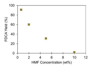
Fig. 12 Effect of initial HMF concentration on final FDCA yields observed in an aqueous system using a Ru/MnO<sub>2</sub> catalyst without the addition of base. Reaction conditions: 2:1 HMF: catalyst weight ratio, T=373 K,  $P_{\rm O_2}=3$  MPa, t=24 h.<sup>25</sup>
