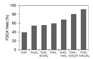
Fig. 14 FDCA yields of various Cu- and Co-based catalysts where G represents graphite deposited catalysts and  $G_P$  represents the PVP-organized catalyst on graphite. All HMF conversions were greater than 95%. Reaction conditions: 0.525:1 HMF: catalyst by wt, 3.2 mmol NaClO, 0.5 mmol HMF, T = 303 K, P = atm, t = 1 h.<sup>95</sup>
