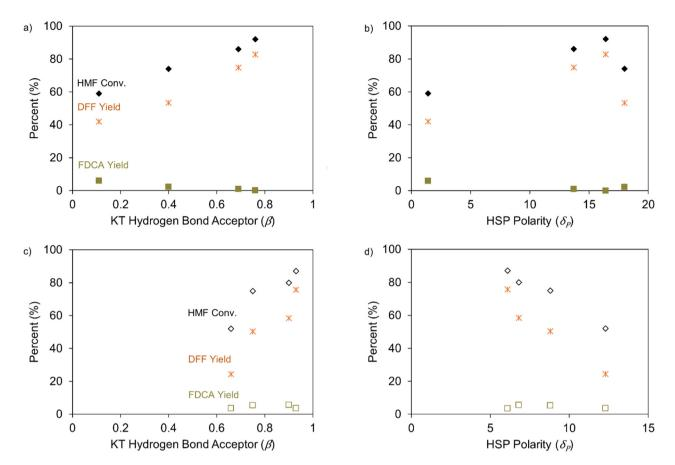
Fig. 25 Trends of HMF conversion (•), DFF (\*), and FDCA (■) yields for toluene, ACN, DMF, and DMSO pure solvents compared to (a) the KT β parameter and (b) the HSP polarity parameter and the same trends for MeOH, EtOH, n-PrOH, and i-PrOH in figure (c) and (d), respectively. Reaction conditions: Co/MnO<sub>2</sub> catalyst, 0.57–0.80 wt% HMF, T = 413 K,  $P_{O_2} = 0.3$  MPa, t = 4 h.<sup>109</sup>
