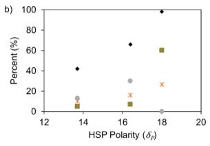
Fig. 24 Effect of solvent (a) hydrogen bond acceptance capacity and (b) polarity on HMF conversion (•) and FDCA (■), DFF (\*\*), and FFCA (•) yields for ACN, DMF, and DMSO solvents. Reaction conditions: CoFeP-400/LDH catalyst, 0.36 mL TBHP oxidant additive, 0.44-0.61 wt% HMF,  $T = 353 \text{ K}, P_{O_2} = 1 \text{ MPa}, t = 6 \text{ h}.^{27}$
