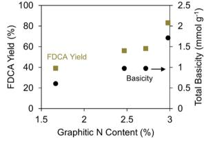
Fig. 22 Impact of graphitic N content on FDCA yield ( ) and total catalyst basicity (●). Reaction conditions: MeOH solvent, 0.1 M K<sub>2</sub>CO<sub>3</sub> weak base additive, 0.89 wt% HMF, T = 433 K,  $P_{O_2} = 2$  MPa, t = 6 h.<sup>23</sup>
