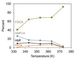
Fig. 8 Remaining HMF (♦) and product yields of FDCA (■), HMFCA (●), and FFCA (A) for a 5.6 wt% Au catalyst on MnO<sub>2</sub>. Reaction conditions: 9.3:1 HMF : catalyst molar ratio, and  $t = 12 \text{ h.}^{65}$
