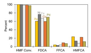
**Fig. 6** Yields and conversion of adding metals to an Au/MgAlO $_x$  catalyst Reaction conditions: 70:1 HMF: metal molar ratio, 0.25 wt% initial HMF, T=363 K,  $P_{\rm O_2}=0.5$  MPa, and t=2 h.  $^{73}$
