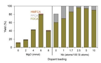
Fig. 11 Impact of dopant amount on FDCA ( $\blacksquare$ ), FFCA ( $\blacksquare$ ), and HMFCA ( $\blacksquare$ ) yields for a MgO dopant loaded on a 4% Ru/Cu1–Co1–O·MgO catalyst (100% HMF conversion for all)<sup>66</sup> and Nb loading on a Ru/SBA-15 catalyst. Reaction conditions:  $P_{O_2}=1$  MPa, t=12 h and for Cu1–Co1–O·MgO catalyst: 0.5 wt% HMF, T=383 K,<sup>66</sup> and for Nb-SBA-15 catalyst: 1.25 wt% HMF, T=393 K.<sup>86</sup>
