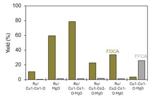
Fig. 9 Support and metal effects on FDCA ( ) and FFCA ( ) yields for HMF oxidation using 4 wt% Ru (when noted) on various Cu, Co, and Mg oxides supports. Reaction conditions: 0.5 wt% HMF, T = 383 K,  $P_{O_0} =$ 1 MPa,  $t = 12 \text{ h.}^{66}$
