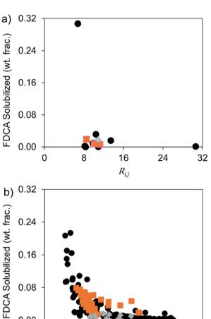
Fig. 16 Relationship between the  $R_{ij}$  parameter and FDCA solubility in (a) pure solvents and (b) binary aqueous/organic mixtures and ternary aqueous/organic/organic mixtures from ( $\bullet$ ),  $^{\bar{3}4}$  ( $_{\bullet}$ ),  $^{108}$  and ( $_{\bullet}$ ).  $^{35}$
