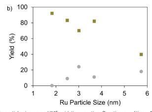
Fig. 18 Comparison of the effect of catalyst (a) metal surface area and (b) Ru particle size on an HMF oxidation reaction. Reaction conditions: 1:1.43 HMF: catalyst by weight, 70/30 w/w water/ACE, 5 wt% initial HMF, T = 383 K,  $P_{O_2} = 1$  MPa, t = 12 h.<sup>53</sup>
