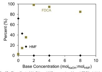
Fig. 15 The effect of NaOH on HMF conversion (\*) and FDCA yield (\*\*) using a Co-Bi oxide catalyst. Reaction conditions: 0.056 HMF: catalyst molar ratio, 0.8 mmol of NaOH, T = 380 K,  $P_{O_2} = 0.6$  MPa, t = 3 h.  $^{97}$
