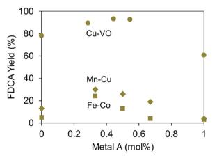
Fig. 19 Comparison of FDCA yields on single metal and bimetallic catalysts containing Mn−Cu (•), Fe−Co (■), 26 and Cu<sup>2+</sup>−VO<sup>2+</sup> over a PVDTA support (•). 113 Reaction conditions for the Mn-Cu and Fe-Co catalysts: 1:4 HMF:catalyst by weight, pure ACN, 13:1 TBHP:HMF molar ratio, 3.5 wt% initial HMF, T = 333 K, P = atm, t = 3 h, t = 3 h, and for the Cu-VO/ PVDTA catalyst: 32/68 w/w DMSO/TBA, 0.37 wt% initial HMF, T = 363 K, P = atm, t = 5 h.<sup>113</sup>
