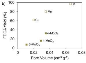
Fig. 20 The relationship between FDCA yield and (a) surface area and (b) pore volume for NNM catalysts on  $\alpha$ -MoO<sub>3</sub> supports ( $\square$ ) and different MoO<sub>3</sub> phases without additional metal (m) (reaction conditions: 4 mL TBA solvent, 4 mmol TBHP, 0.4 wt% HMF, T = 353 K, P = atm, t = 12 h). 50
