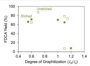
Fig. 13 The effect of graphitization on FDCA yields. Reaction conditions: 0.024 HMF: catalyst molar ratio, T=338 K,  $P_{\rm O_3}=0.5$  MPa, t=12 h.  $^{94}$
