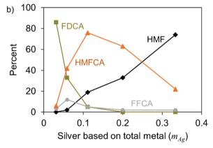
Fig. 7 Effect of silver loading on a bimetallic (a) Au/Ag SiO<sub>2</sub> catalyst (conditions: 79:1 HMF:Au molar ratio, 0.4 mmol NaHCO<sub>3</sub>, T=353 K,  $P_{\rm O_2}=1$  MPa, and t=6 h)<sup>68</sup> and (b) Pt/Ag catalyst where the *x*-axis represents the mass fraction of Ag of the total mass of the metals. Reaction conditions: 50:1 HMF:Pt molar ratio, 0.8 mmol NaHCO<sub>3</sub>, T=373 K, O<sub>2</sub> bubbling at 75 mL min<sup>-1</sup>, and t=1 h.<sup>60</sup>
