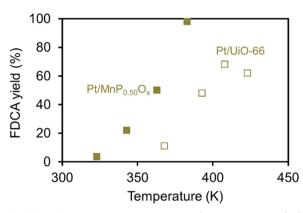
Fig. 4 Effect of reaction temperature on FDCA yield with a Pt/UiO-66 catalyst ( $\square$ )<sup>74</sup> and a Pt/MnP<sub>0.50</sub>O<sub>x</sub> catalyst ( $\square$ ).<sup>58</sup> Reaction conditions for Pt/UiO-66 catalyst: HMF: Pt 200:1 molar ratio,  $P_{\rm O_2}$  = 0.5 MPa, t = 14 h<sup>74</sup> and for Pt/MnP<sub>0.50</sub>O<sub>x</sub> catalyst: HMF: Pt 100:1 molar ratio,  $P_{\rm O_2}$  = 1 MPa, t = 24 h<sup>58</sup>
