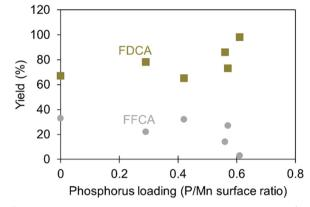
Fig. 3 Impact of P dopant amount on the surface of the catalyst (determined by XPS) on FDCA (■) and FFCA (■) yields for MnP<sub>v</sub>O<sub>x</sub> catalyst (100% HMF conversion for all). Reaction conditions: 100:1 HMF: Pt molar ratio, 1.25 wt% HMF, T = 383 K,  $P_{\rm O_2}$  = 1 MPa, 24 h. <sup>58</sup>
