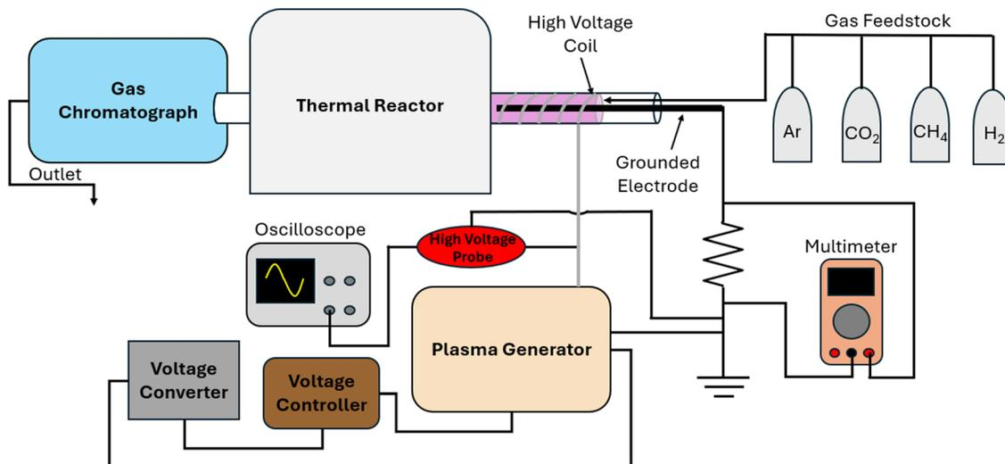
Fig. 1 Diagram of plasma-thermal tandem reactor setup.
