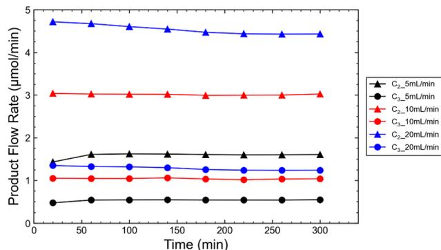
**Fig. 3** Effect of total flow rate on C<sub>2</sub> (▲) and C<sub>3</sub> (●) species production. C<sub>2</sub> species included C<sub>2</sub>H<sub>4</sub> and C<sub>2</sub>H<sub>6</sub> while C<sub>3</sub> species included C<sub>3</sub>H<sub>6</sub> and C<sub>3</sub>H<sub>8</sub>. Total flow rate was specified next to each dataset.
