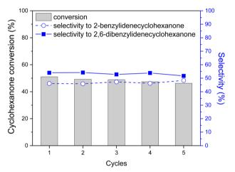
Fig. 6 Catalytic activity of the  $Nb_2C$  MXene sample after 5 cycles in the condensation of cyclohexanone with benzaldehyde. Reaction conditions: cyclohexanone 1 mmol, benzaldehyde 2 mmol, catalysts 20 mg, no solvent, reaction temperature 120 °C, magnetic stirring at 500 rpm, and time 2 lb.
