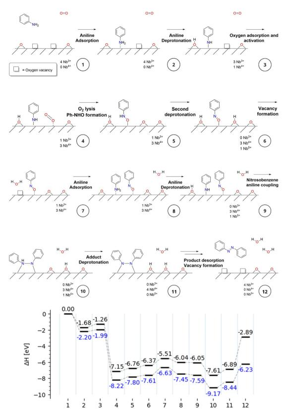
Fig. 7 Proposed reaction mechanism of the aniline oxidative coupling reaction with Nb<sub>2</sub>CO<sub>2</sub> MXene as the catalyst (top). Reaction energy profile of the reaction intermediates provided by CASTEP DFT (black) and Matlantis (blue) codes (bottom).
