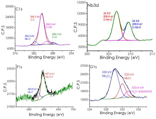
Fig. 2 High-resolution XPS peaks of the elements detected in Nb<sub>2</sub>C MXene, showing the best deconvolution for each spectrum into the individual components whose assignment, binding energy and contribution percentage are indicated in the plot.
