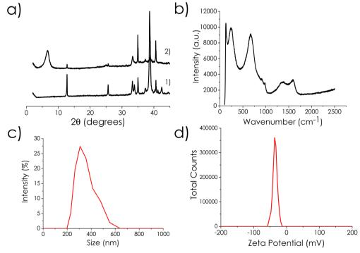
Fig. 1 (a) XRD spectra of Nb<sub>2</sub>AlC (1) and Nb<sub>2</sub>C MXene (2) after Al etching. (b) Raman spectrum of Nb<sub>2</sub>C MXene recorded with a 413 nm excitation. (c) Dynamic laser scattering of aqueous suspensions of Nb<sub>2</sub>C MXene (1 mg mL $^{-1}$ ). (d) Zeta potential of aqueous Nb<sub>2</sub>C MXene suspension at neutral pH.
