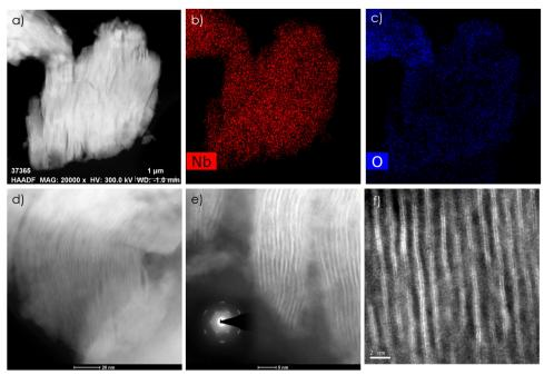
Fig. 3 TEM images of the Nb<sub>2</sub>C MXene sample under study, showing the 2D morphology at four magnifications (a), (d), (e) and (f), and the Nb (b) and O (c) distribution mappings of Fig. 3a. The inset of Fig. 3e shows high crystallinity of the Nb<sub>2</sub>C sheets.
