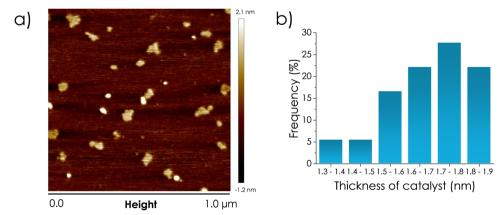
Fig. 4 (a) Frontal view of the Nb<sub>2</sub>C MXene sample on an atomically flat mica. (b) Vertical profiles along ten different particles, showing a modal thickness value in the range 1.7-18 nm.
