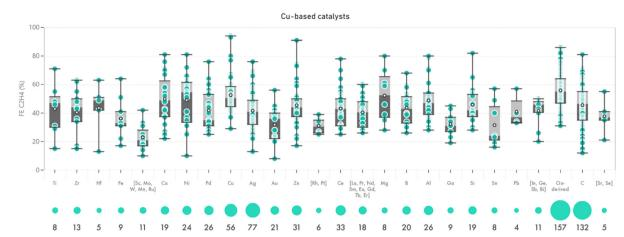
Fig. 1 High-level overview of the catalyst systems compiled in this work, depicting the maximum C<sub>2</sub>H<sub>4</sub> FE distribution for the catalyst systems as grouped based on their elemental composition, together with the number of sources identified for each of these categories
