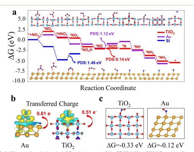
Fig. 4 (a) Free-energy diagram for electrochemical NO<sub>3</sub><sup>-</sup> reduction to ammonia (NH<sub>3</sub>) on TiO<sub>2</sub>(110), Au(111), and Si(111) (b) Charge-density difference for Au(111) and TiO<sub>2</sub>(110), where the yellow and cyan colours depict charge accumulation and charge depletion, respectively. (c) Adsorption free-energy changes of NO(g) to \*NO on TiO<sub>2</sub>(110) and Au(111). Colour code, Ti: light blue, Au: gold, O: red, N: blue, H: white.
