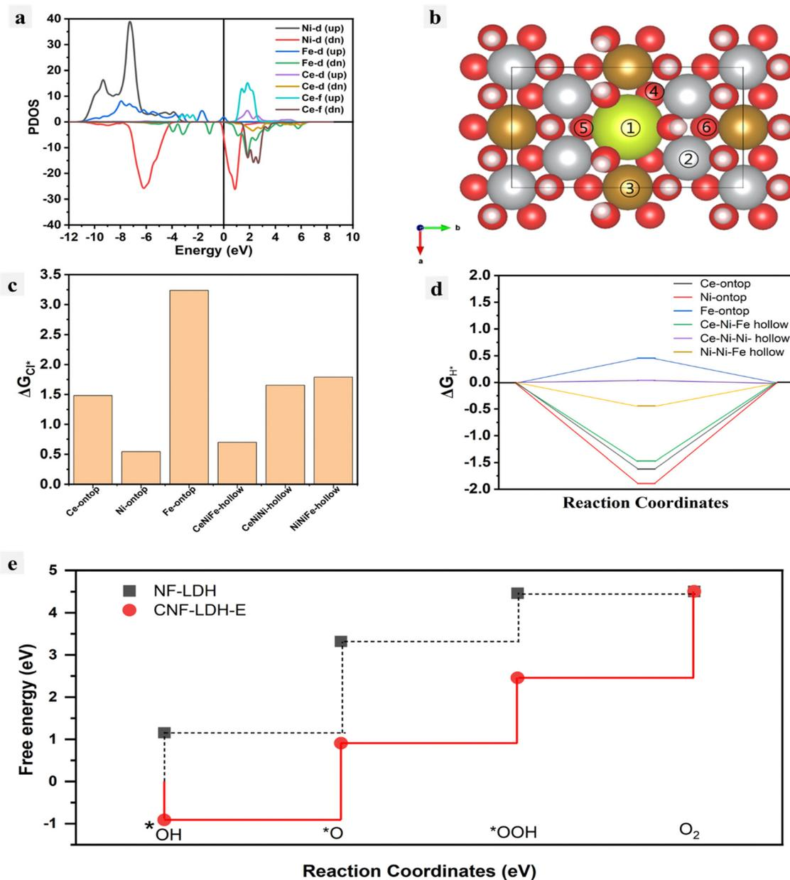
**Fig. 6** DFT calculations on the CNF-LDH-E. (a) PDOS plot of the CNF-LDH-E, (b) theoretical model showing the adsorption sites for the adsorption of  $Cl^*$ , free energy calculation for the (c)  $Cl^*$  adsorption and (d)  $H^*$  adsorption and (e) free energy calculations for the different intermediate involved in OER for NF-LDH and NF-LDH-E.
