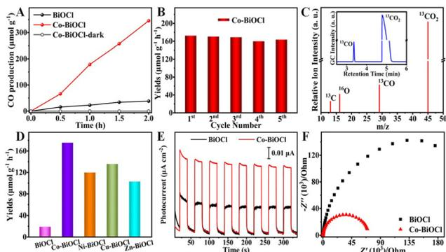
Fig. 2 (A) Photocatalytic CO<sub>2</sub> activities of as-prepared photocatalysts. (B) Cycling tests of Co-BiOCl sample. (C) Mass spectrum of the <sup>13</sup>CO<sub>2</sub> photoreduction products over Co-BiOCl (inset image: GC signal). (D) Comparative presentation of CO evolution rates. (E) *i*-*t* curves and (F) EIS curves of the as-obtained photocatalysts.
