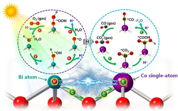
**Scheme 1** Schematic diagram of the neighboring effect for CO<sub>2</sub> photo-reduction over the Co-BiOCl sample.
